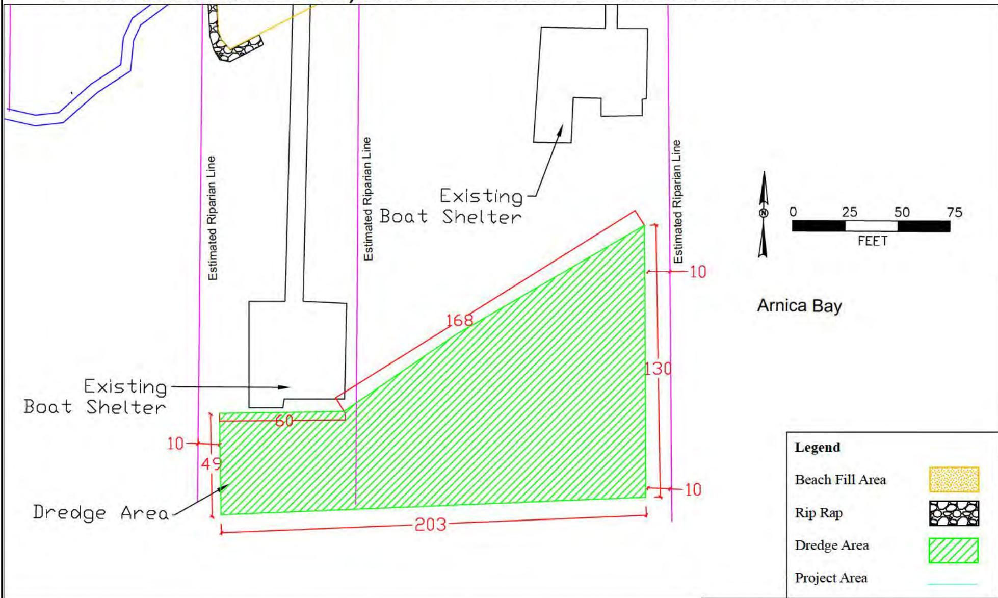
Note: All dimensions shown are measured in feet. Drawings are for USACE, ADEM and AL State Lands permitting only and should not be used for construction.
