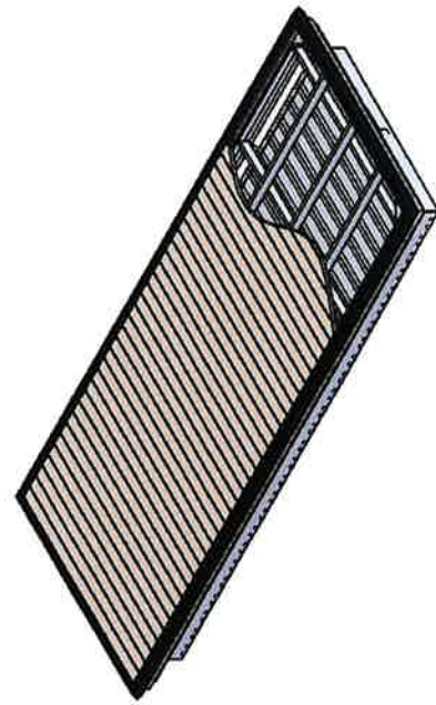
ISOMETRIC VIEW OF ALUMINUM TOP DECKED FULL FLOATING DOCK SCALE: NTS
