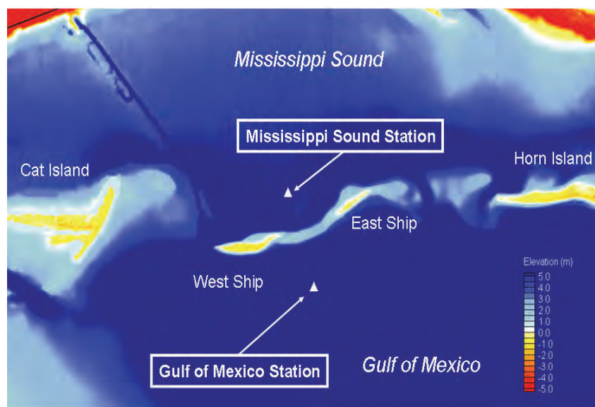
Figure 7-2. Location map showing the two 2010 ERDC wave gauge deployment locations near Ship Island (from Chapter 4).
