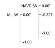
ELEVATION CONVERSION FOR DAUPHIN ISLAND CAUSEWAY DEEPENING AND WIDENING PLACEMENT AREA
