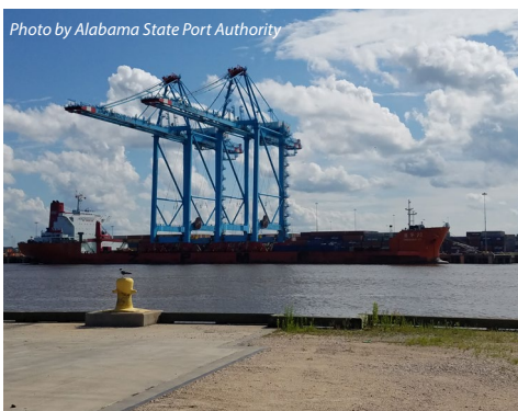
Photo by Alabama State Port Authority Now a permanent part of Mobile's skyline, these new Super Post-Panamax Ship-to-Shore cranes support the growing size of container vessels arriving at Mobile Harbor.
