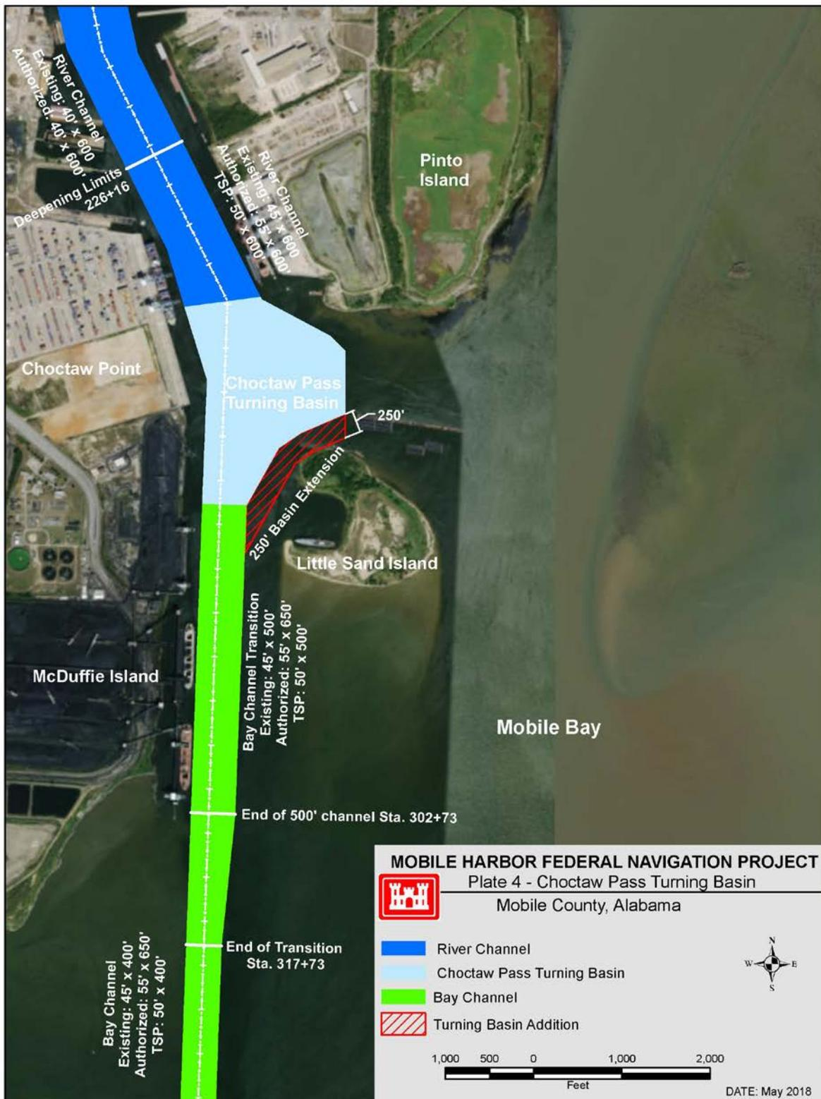
**FIGURE 3.6: CHOCTAW PASS TURNING BASIN EXPANSION**
