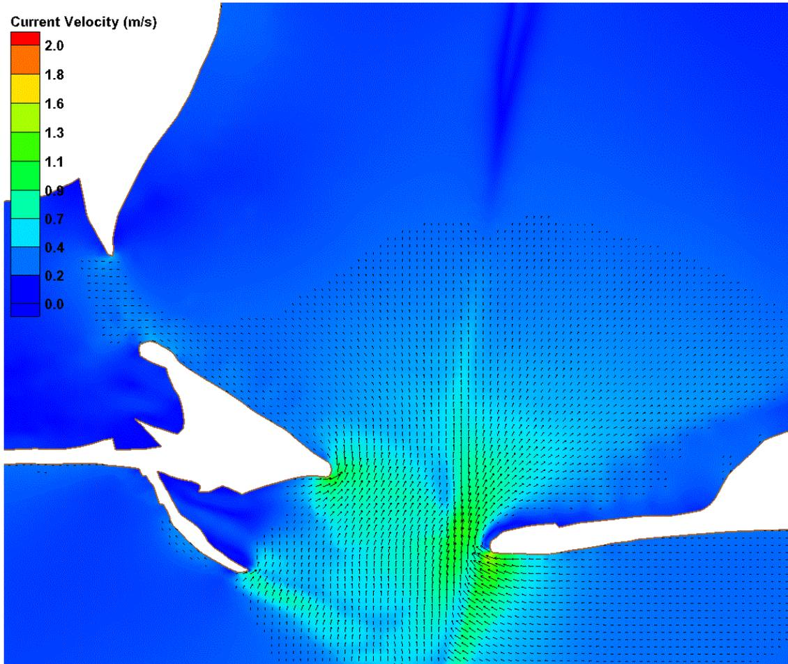
Figure 62. Maximum BEPL SE Flood Current Velocities
