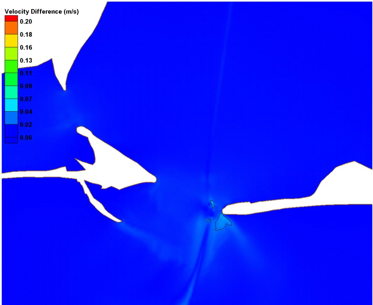
Figure 63. Maximum BEPL SE Flood Current Difference
