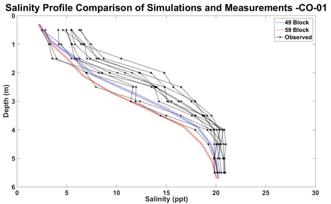
Figure 36. September 13-14, 2016 Observed and Model Salinity Profiles CO-01
