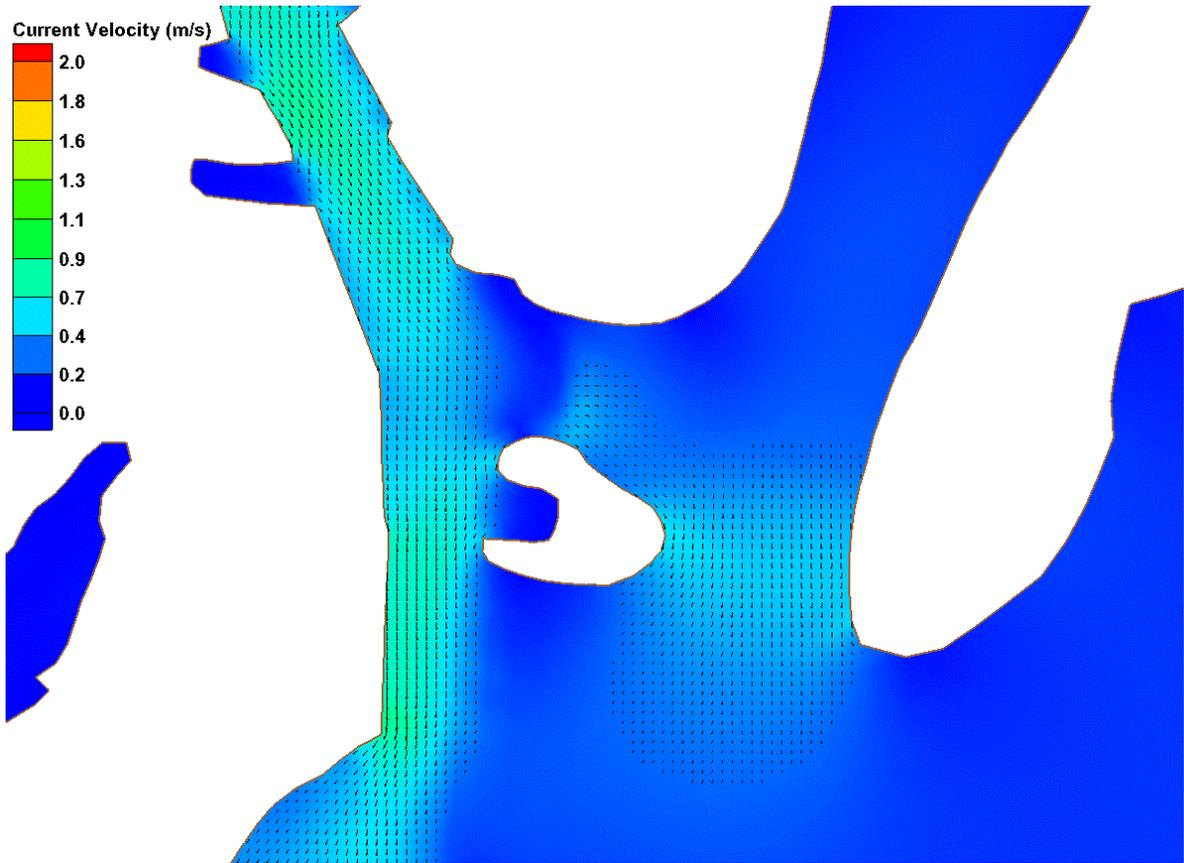
Figure 64. Maximum TB SE Flood Current Velocities
