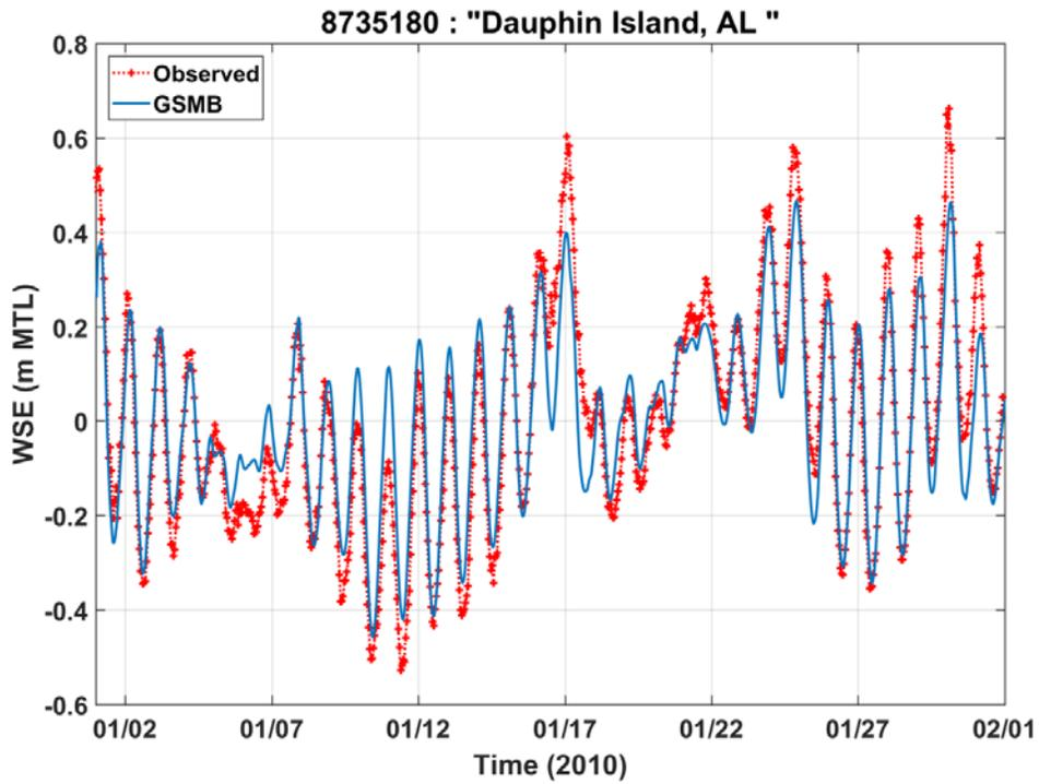
Figure 12. January Dauphin Island Water Surface Elevation Comparison
