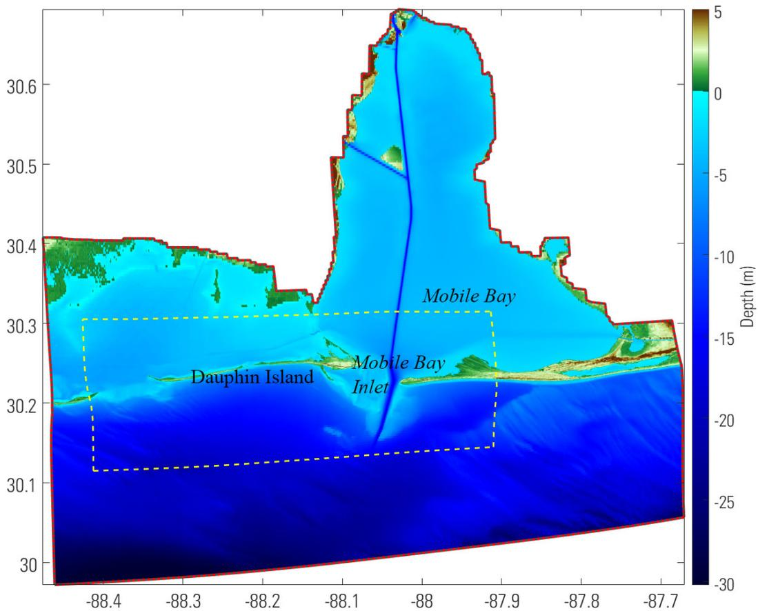
Figure 2. Delft3D model domains (computational grid extents) and initial elevations (existing condition), Mobile Harbor, Alabama. Red dotted line shows the extent of the coarse outer WAVE module grid, grey dotted line shows the extent of the FLOW module grid (which is the same as the coarse outer WAVE module grid), yellow dotted line shows the extent of the nested fine WAVE module grid.
