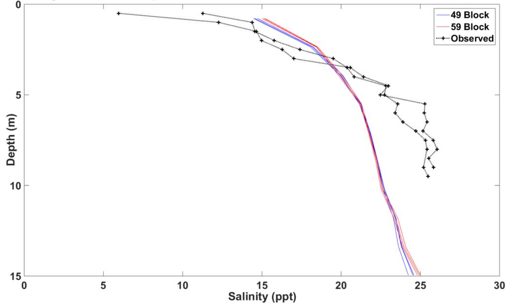
Figure 37. September 13-14, 2016 Observed and Model Salinity Profiles MR-09
