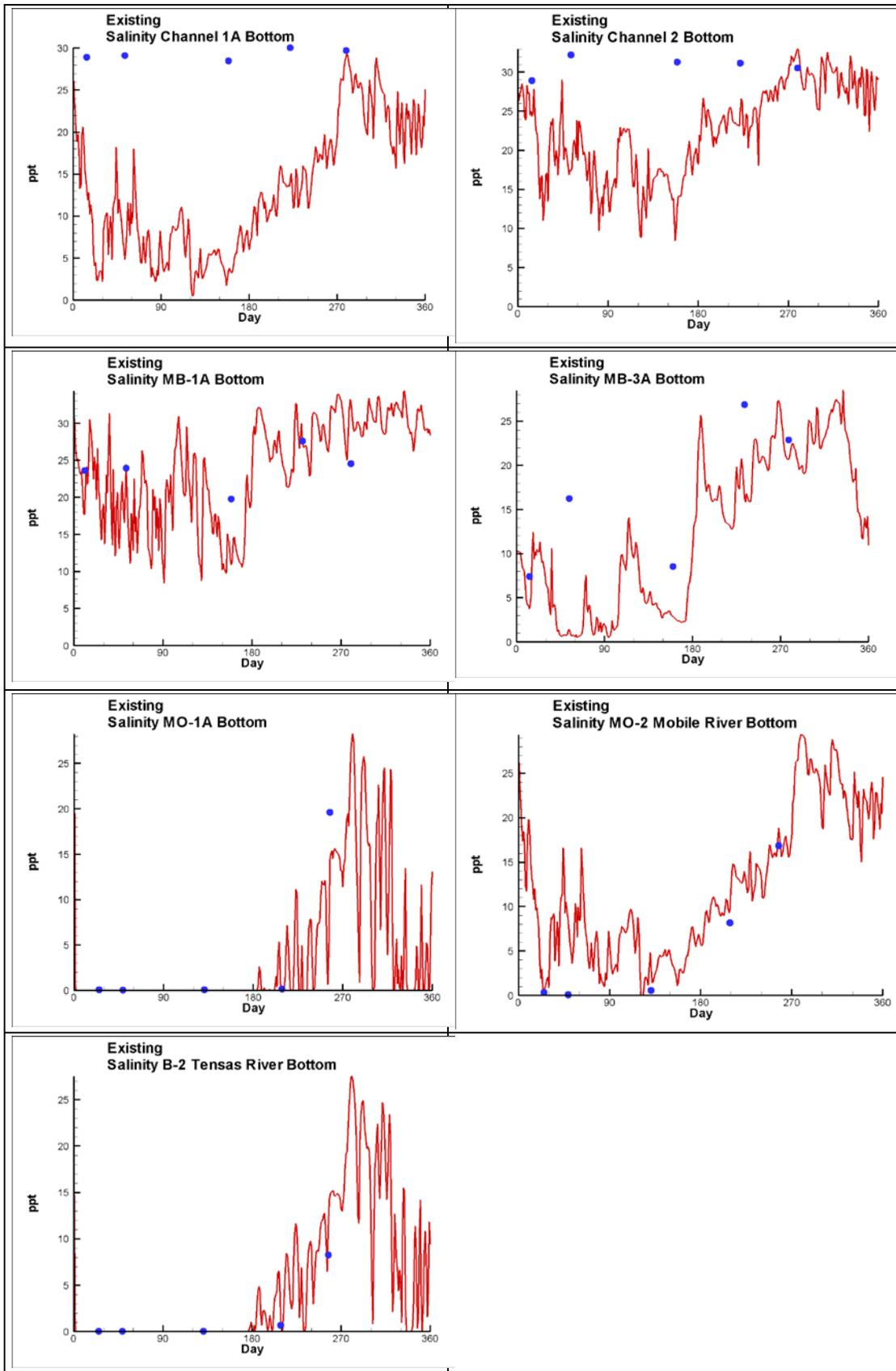
Figure 75. Comparison of Simulated and Measured Bottom Salinities
