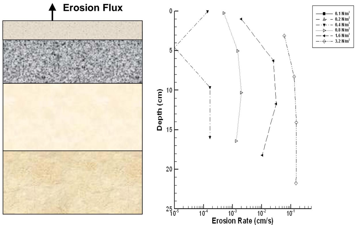
Figure 96. Multi-Bed Layer Model used in GSMB-SEDZLJ
