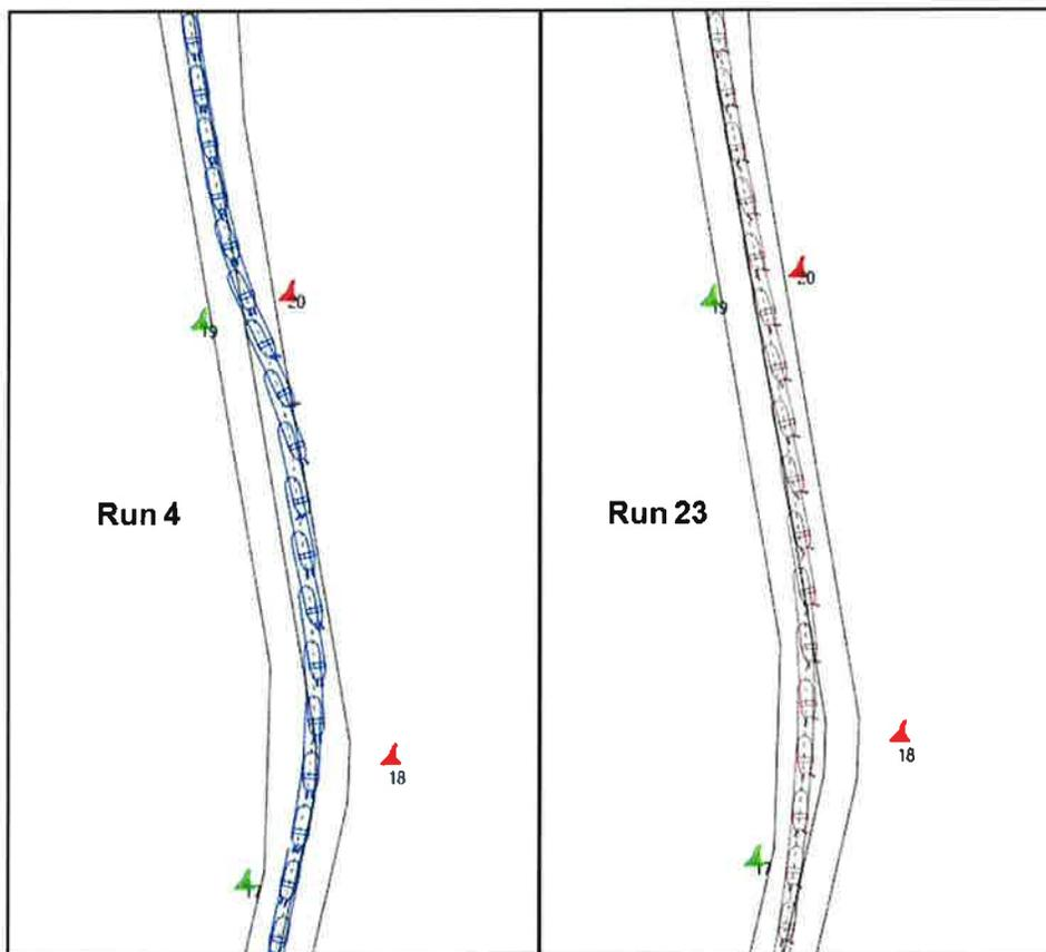
Figure 4. Bend easing impact on inbound vessel transit
