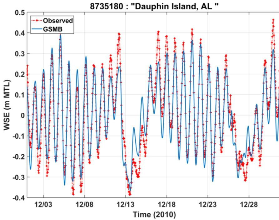
Figure 14. December Dauphin Island Water Surface Elevation Comparison
