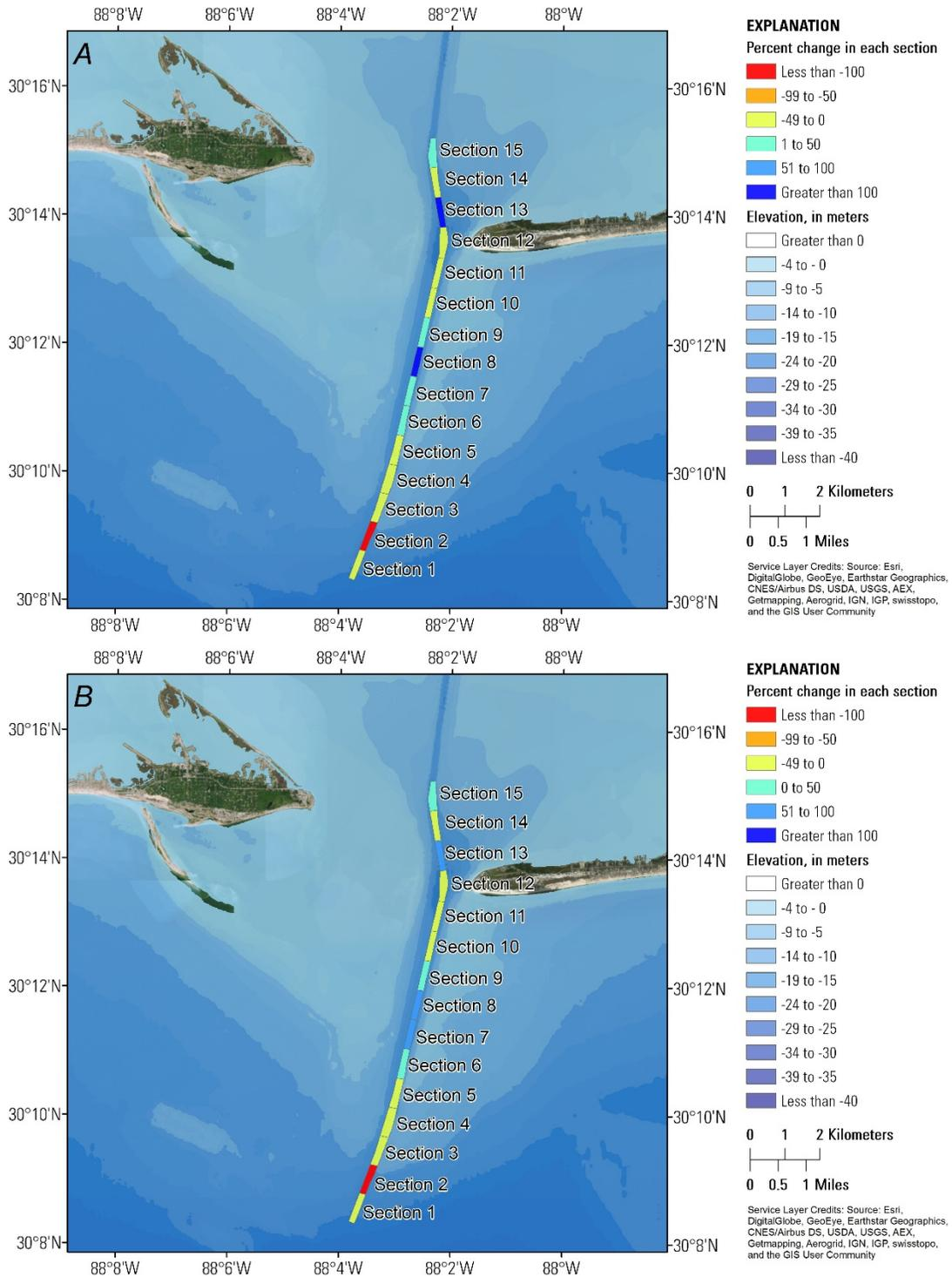
Figure 10. Percent change in the volume of sediment eroded or deposited in the entrance channel, Mobile Harbor, Alabama. A, between the 10-year existing and 10-year with-project conditions. B, between the 10-year existing with 0.50 meter of sea level rise and 10-year with-project with 0.50 meter of sea level rise.
