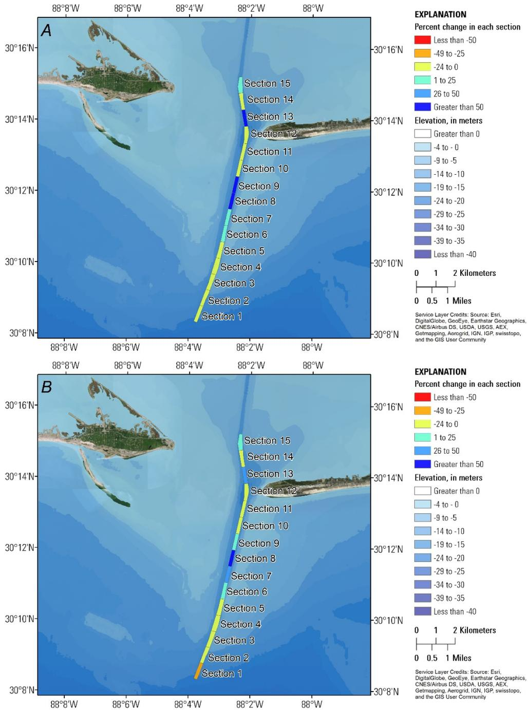
**Figure 7.** Percent change in the volume of sediment eroded or deposited in the entrance channel, Mobile Harbor, Alabama. *A*, between 2010 existing and 2010 with-project conditions. *B*, between 2010 existing with 0.50 meter of sea level rise and 2010 with-project with 0.50 meter of sea level rise.
