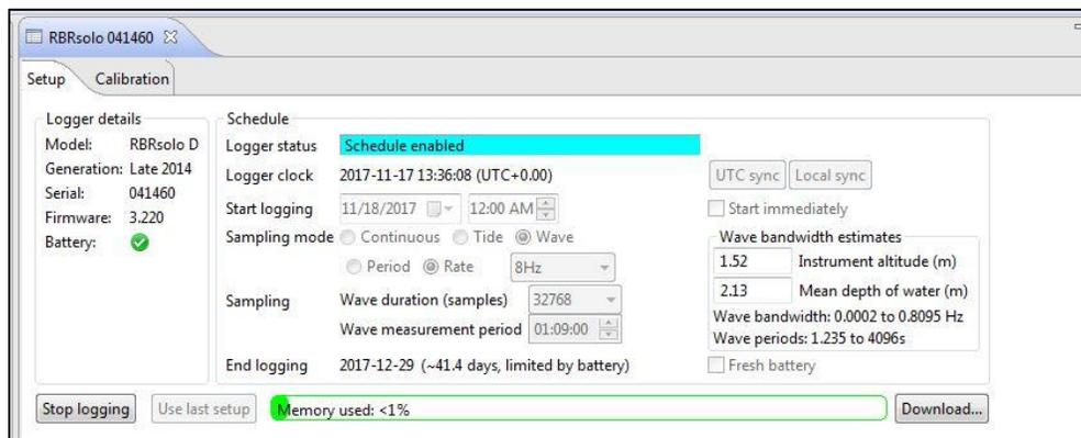
Figure 7: Typical Pressure Sensor Setup
