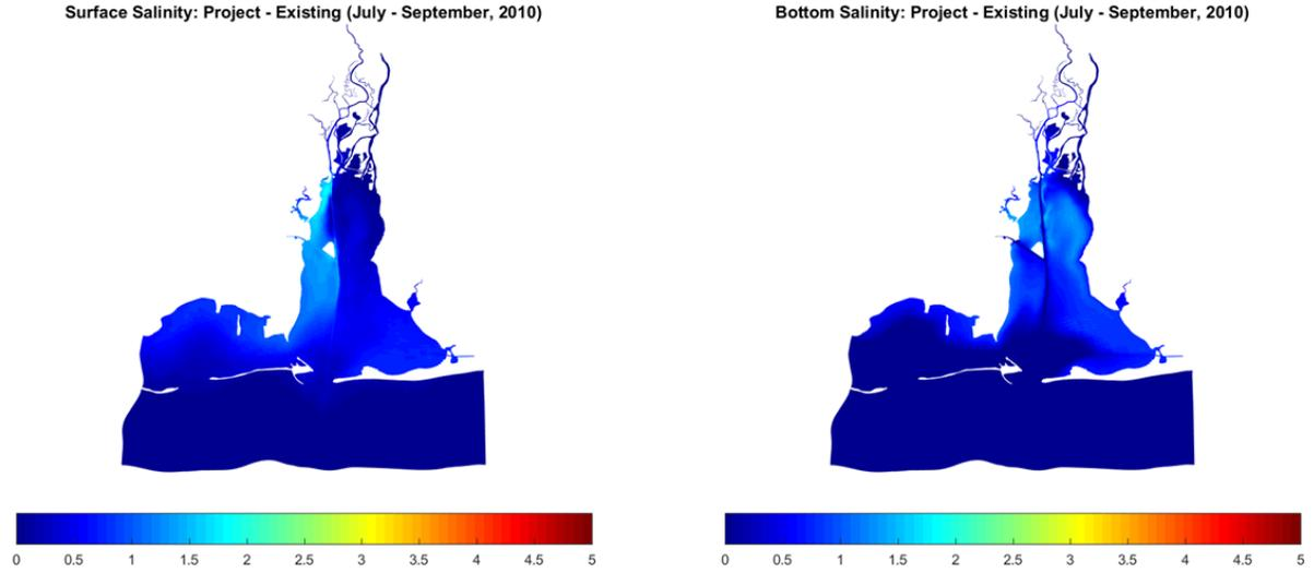
Figure 61. Differences in Surface and Bottom Salinity: July – September 2010
