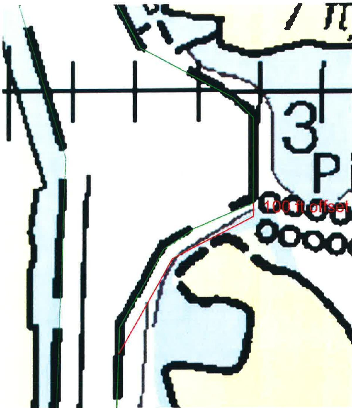
The ships tested on simulator demand an aggressive approach into basin + execution of turn. (in standard Environmentals). Committing to the East side of basin requires extremely close proximity to North + South boundaries. It is not feasible to turn an 1,100' ship that deep in basin without more room for bow to fall South, if another ship docked @ South end of Container Terminal.
