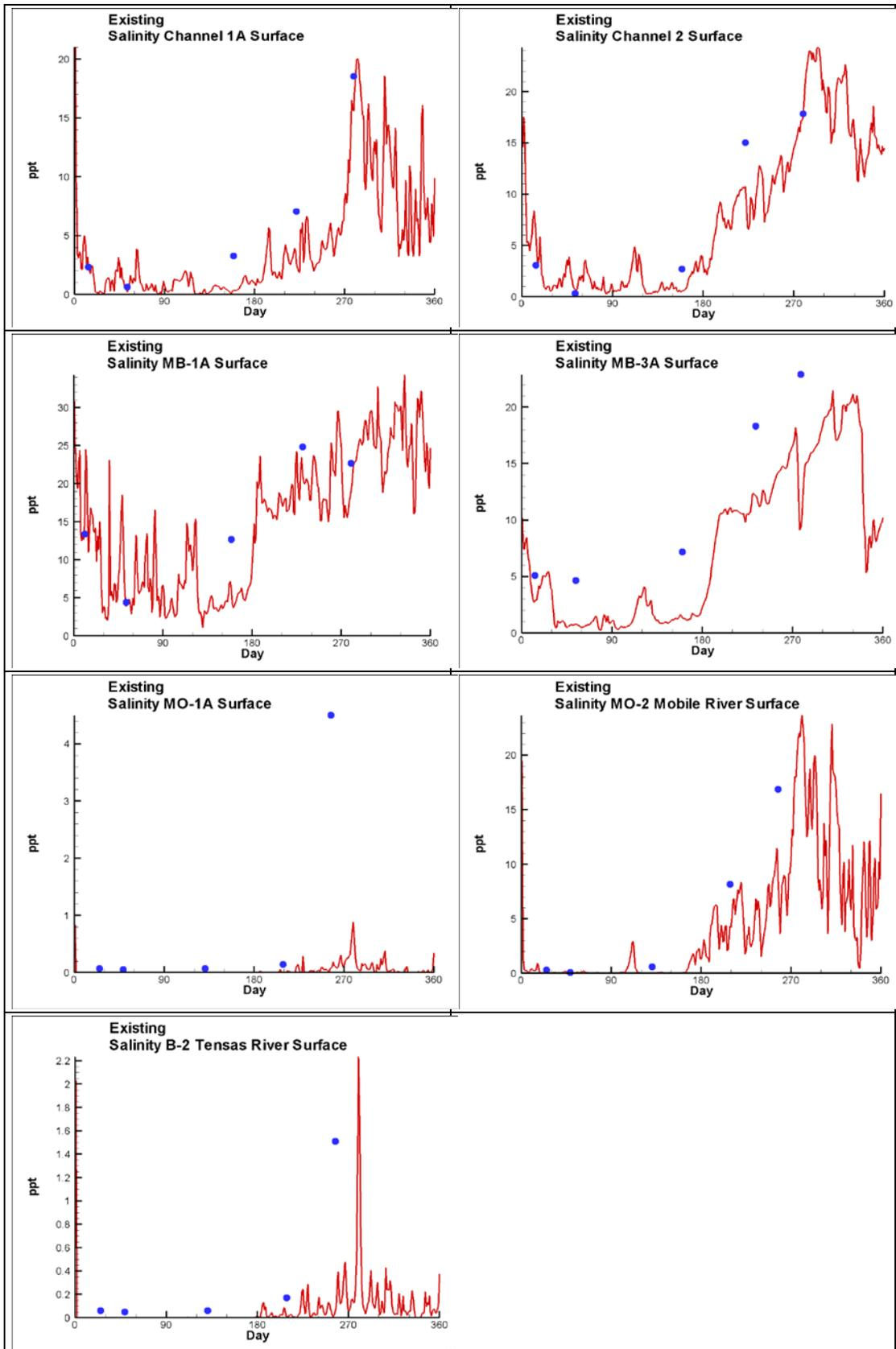
Figure 74. Comparison of Simulated and Measured Surface Salinities
