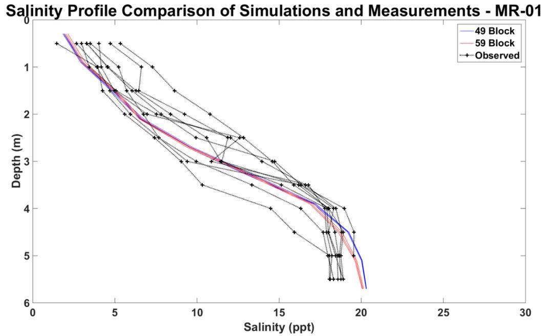
Figure 35. September 13-14, 2016 Observed and Model Salinity Profiles MR-01
