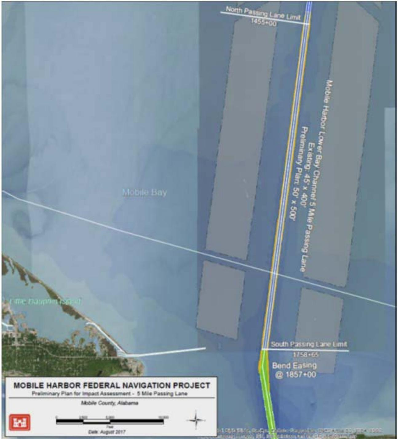
Figure 44. Channel Widening - Passing Lane Design
