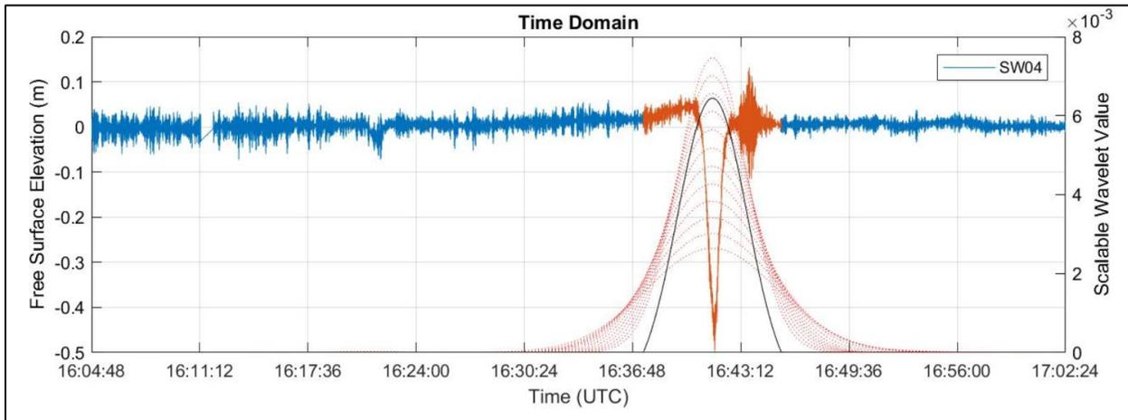
Figure 12: Ideal case of CWT used for automatic identification of a vessel generated disturbance at Station SW04, Event ID: 259 for an inbound traveling vessel with dimensions of  $L = 229$  m,  $B = 32$  m,  $D = 13.7$  m. The orange highlighted area is the signal assumed to be generated by the vessel.
