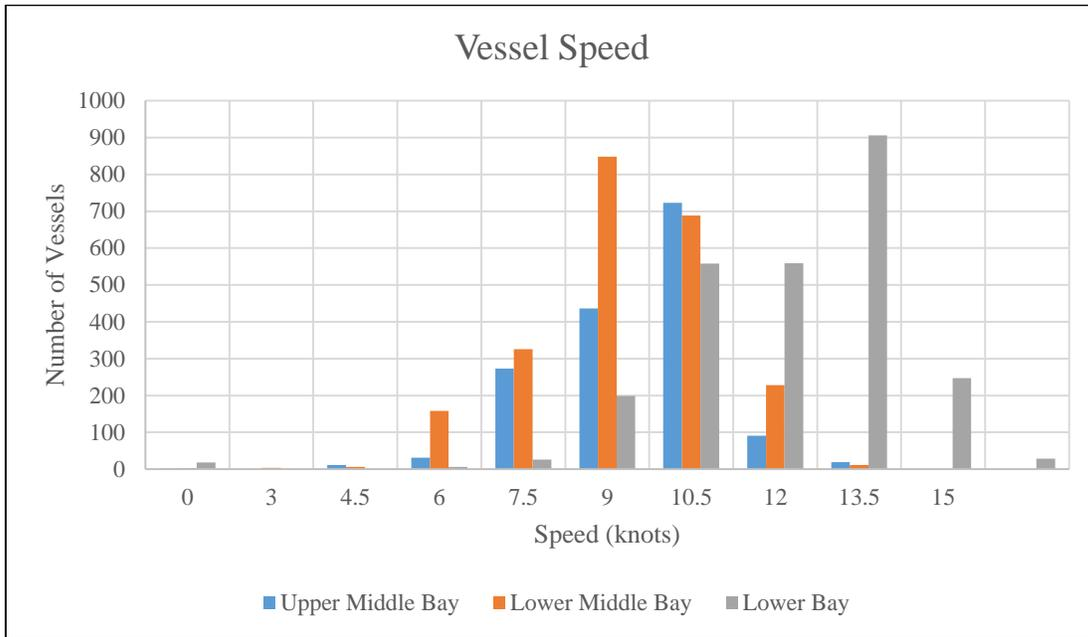
Figure 31: Variation of vessel speed for all classes and categories in Mobile Bay, Alabama with respect to three locations of interest.
