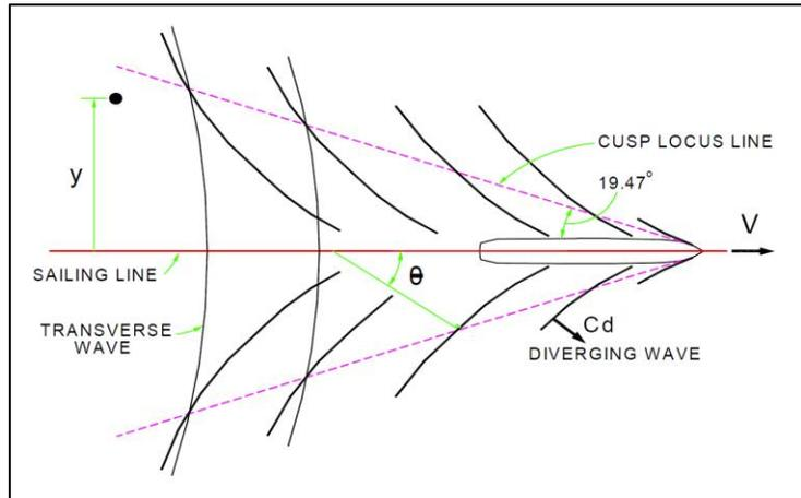
Figure 5: Definition sketch of vessel disturbance in plan-form described by Havelock (1908).
