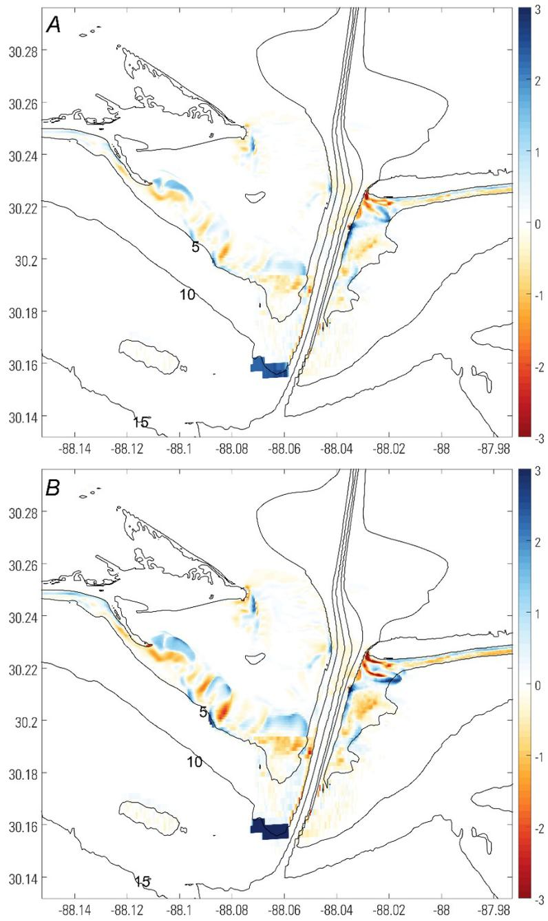
Figure 4. Modeled bed level change in Mobile Harbor, Alabama. *A*, after 10 years in the 10-year existing condition simulation. *B*, after 5 years in the 10-year existing condition simulation. Differences greater than 0 indicate accretion, differences less than 0 indicate erosion.
