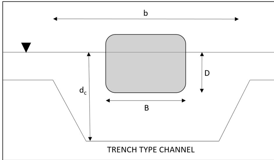
Figure 32: Graphical sketch defining cross-sectional variables used in VGWE and vessel speed computations.
