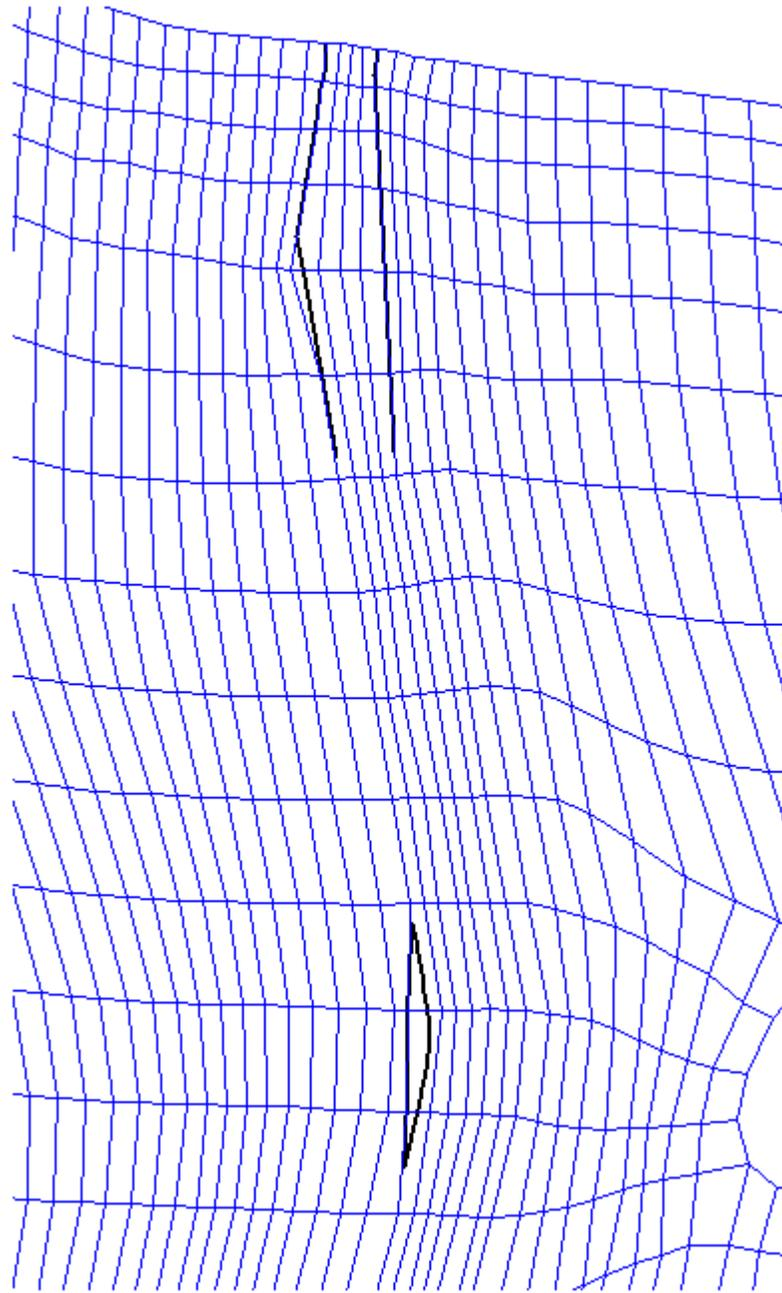
Figure 43. Bend Easing Grid Modification Mobile Bay Entrance
