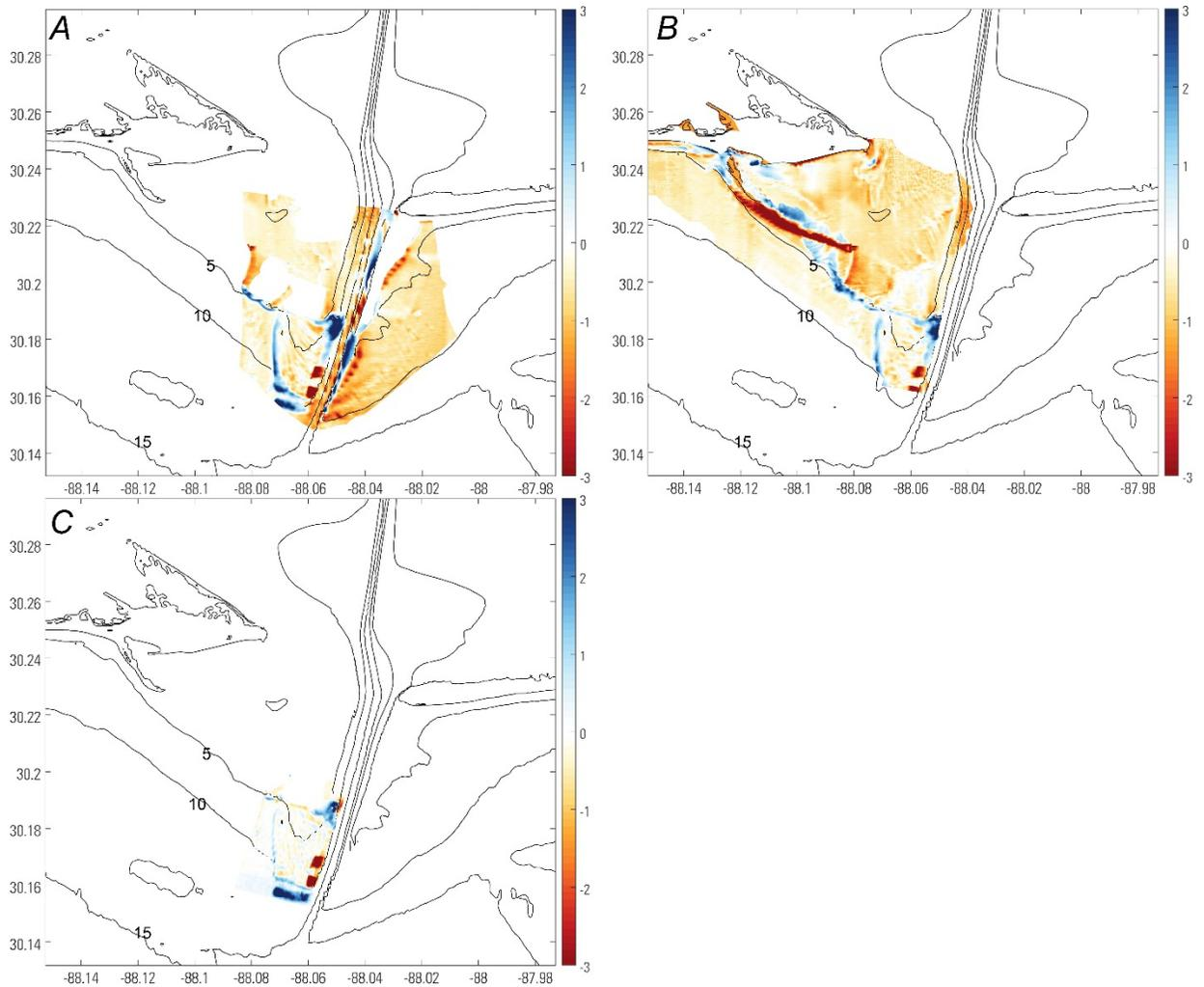
Figure 3. Observed bed level changes in Mobile Harbor, Alabama. *A*, from 2002 to 2014. *B*, from 2002 to 2015. and *C*, from 2009 to 2014. Differences greater than 0 indicate accretion, differences less than 0 indicate erosion. The range of uncertainty is  $\pm 0.61$  m.
