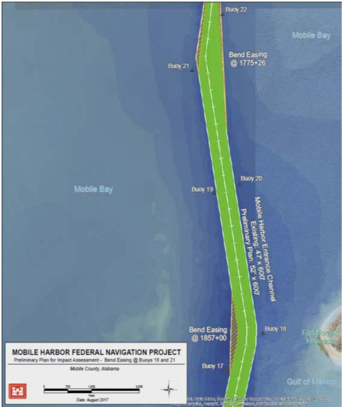
Figure 42. Bend Easing Design at the Mobile Bay Entrance
