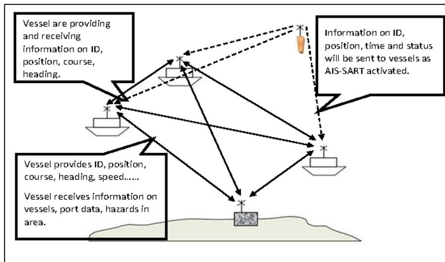
Figure 10: Automatic Information System (AIS) System Schematic. (IMO, 2015)
