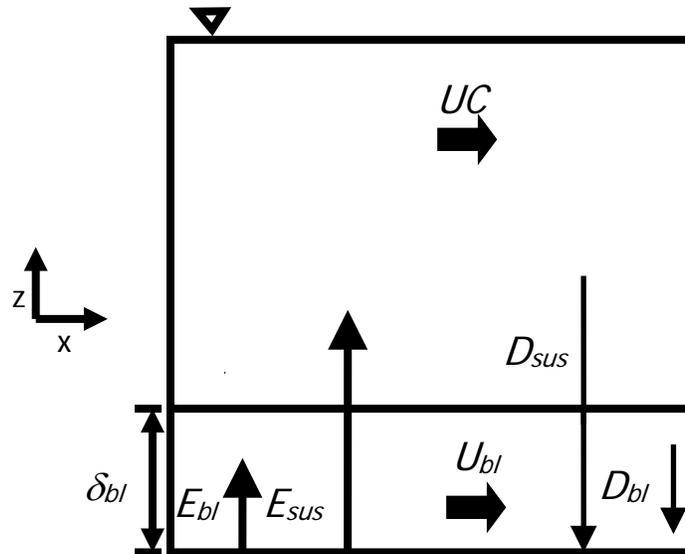
Figure 95. Sediment transport processes simulated in GSMB-SEDZLJ
