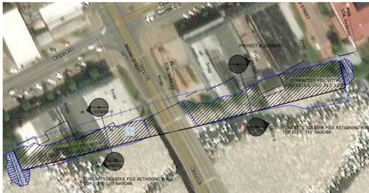
Figure 31: Site Plan for Bank Stabilization
