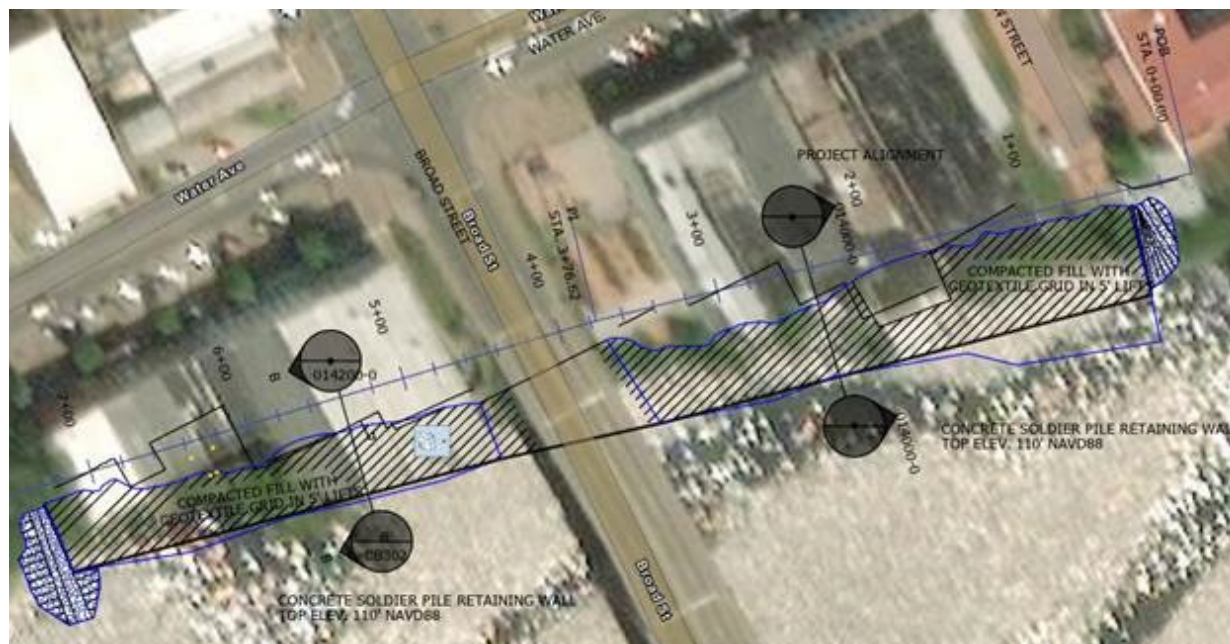
Figure 31: Site Plan for Bank Stabilization
