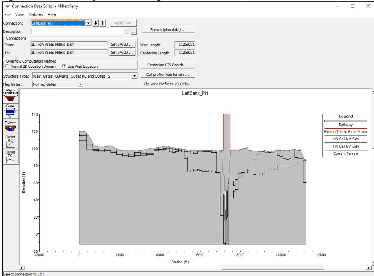
**Figure H.40: Millers Ferry Powerhouse within SA/2D Connection Editor**
