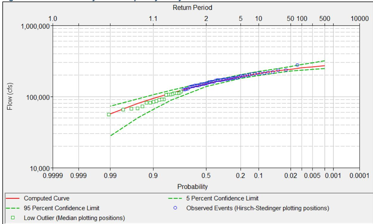
**Figure H.33: Claiborne Flow Frequency Analysis**
