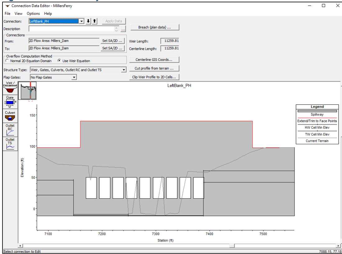
**Figure H.41: Millers Ferry Gated Spillway and Right Descending Bank within SA/2D Connection Editor**
