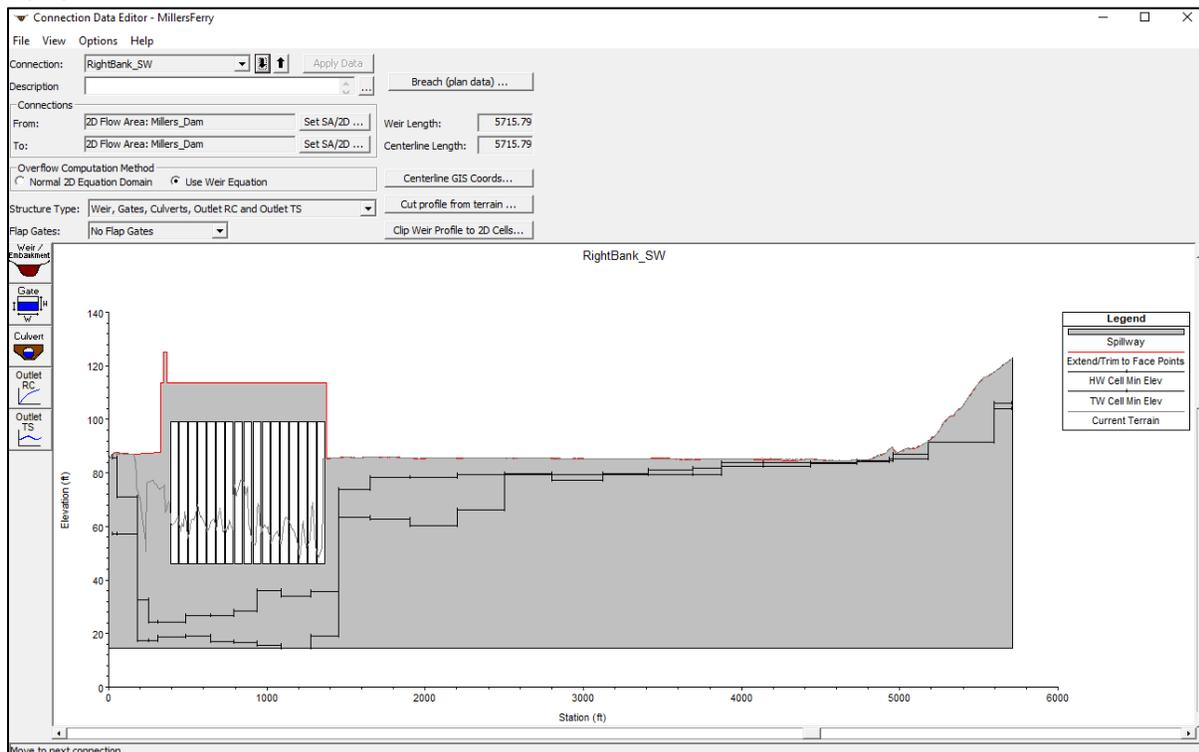
**Figure H.42: Claiborne Spillway within SA/2D Connection Editor**
