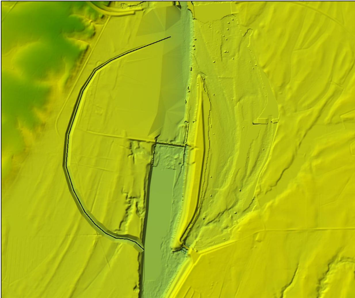
**Figure H.48: Modified Terrain for Claiborne Lock and Dam Right Bank Natural Bypass Channel**
