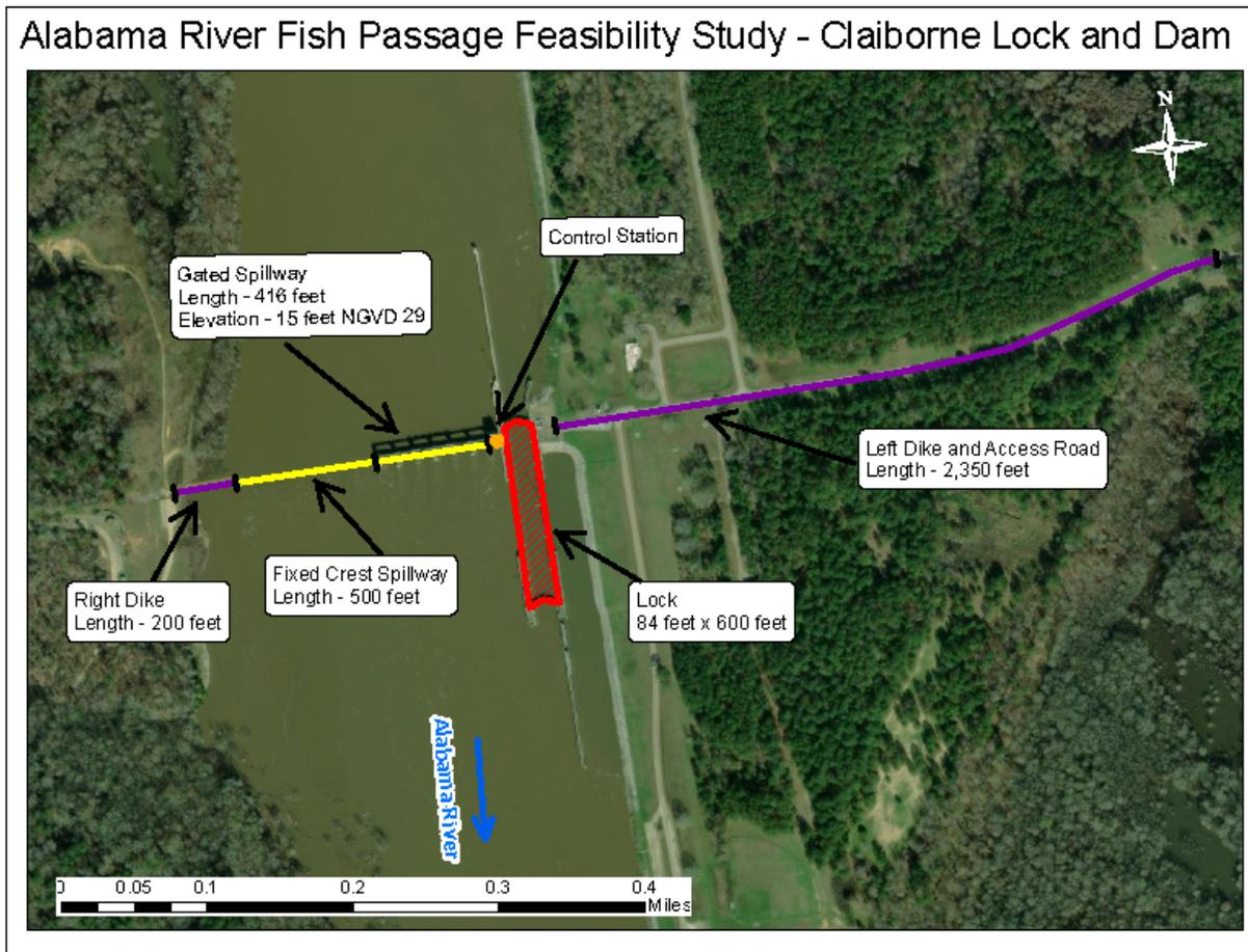
**Figure 2: The Claiborne Lock and Dam**
