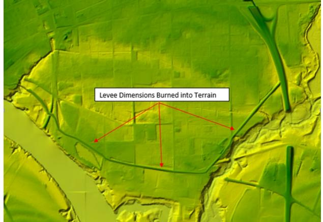
Figure A-61: Image depicting the burned in levee alignment for the L3 Optimized Levee
