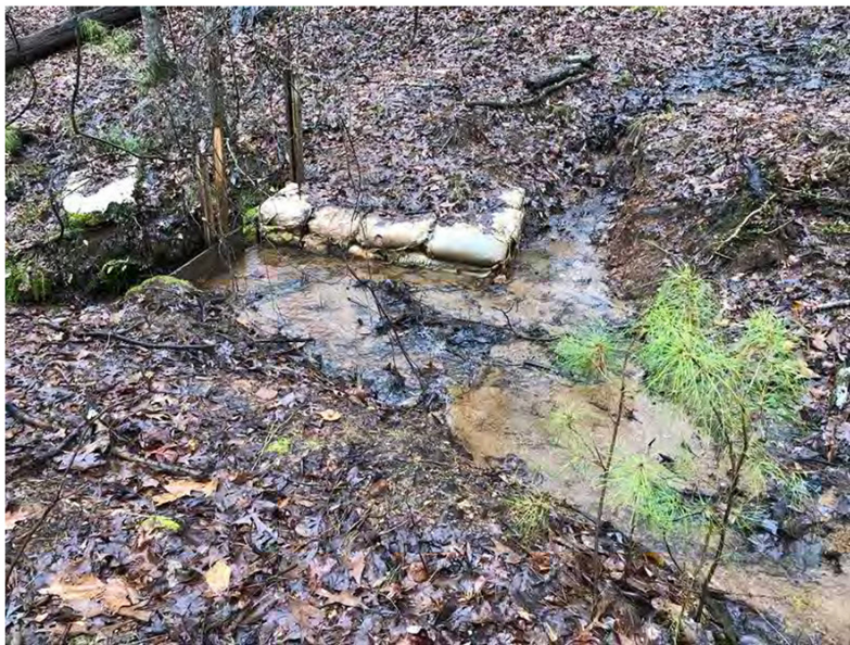
Figure 5 Weir 2, D/S of SD2; flow depth of 1 7/8 inches.
