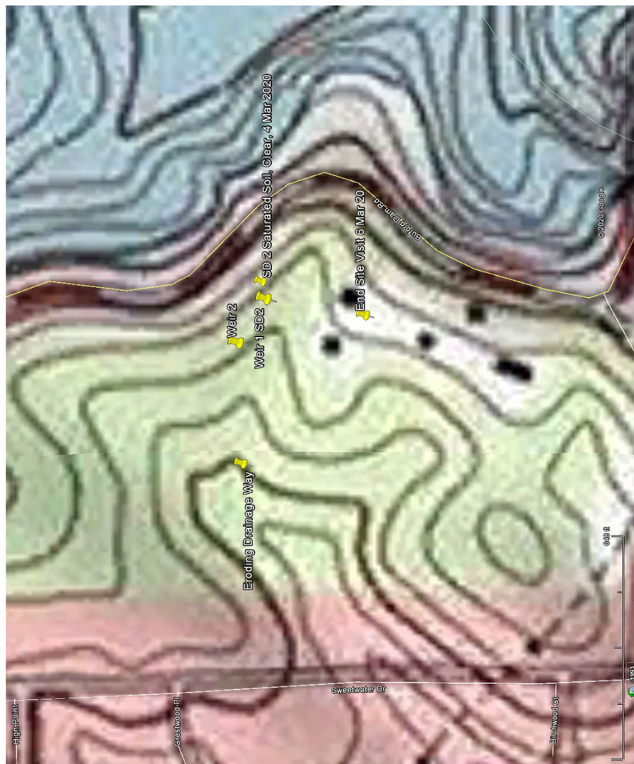
Figure 10 Enlargement of Saddle Dike 2 area on the south and features of note. The Main Dam is depicted on the upper right edge of the map. Contour elevation of the bold contour marked with "Eroding Drainage Way" is 1000 ft. Contour interval is 20 ft.
