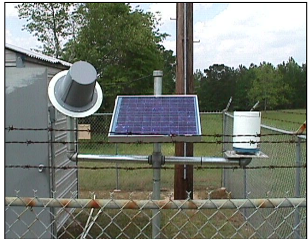
Figure 5-2. Typical Field Installation of a Precipitation Gage
