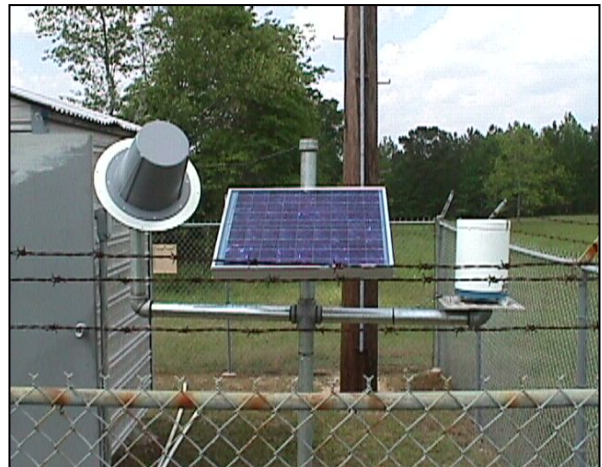
Figure 5-2. Typical Field Installation of a Precipitation Gage
