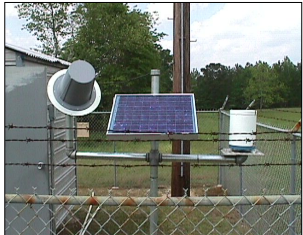
Figure 5-2. Typical Field Installation of a Precipitation Gage
