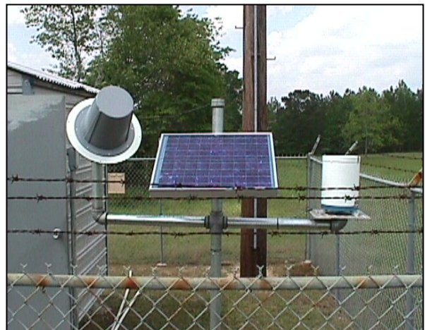
Figure 5-2. Typical Field Installation of a Precipitation Gage
