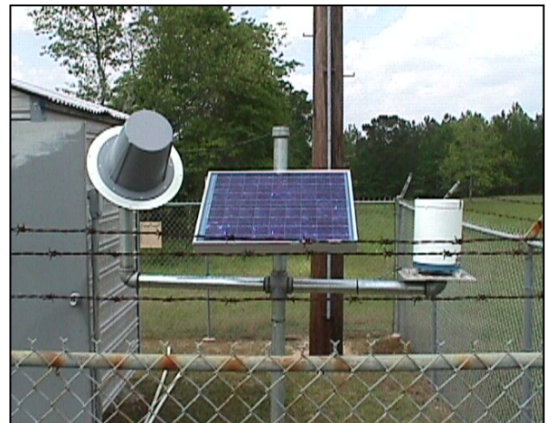
Figure 5-2. Typical Field Installation of a Precipitation Gage
