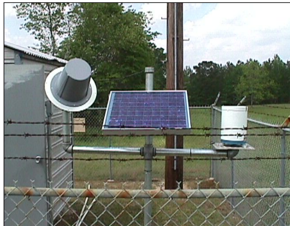
Figure 5-2. Typical Field Installation of Precipitation Gage
