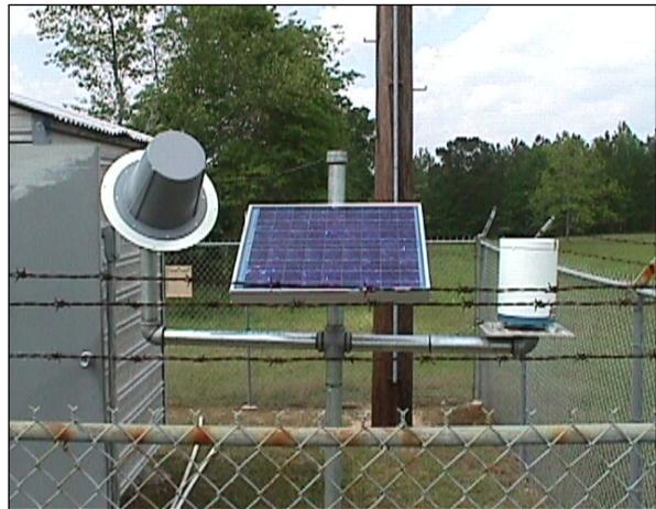
**Figure 5-2. Typical Field Installation of Precipitation Gage**
