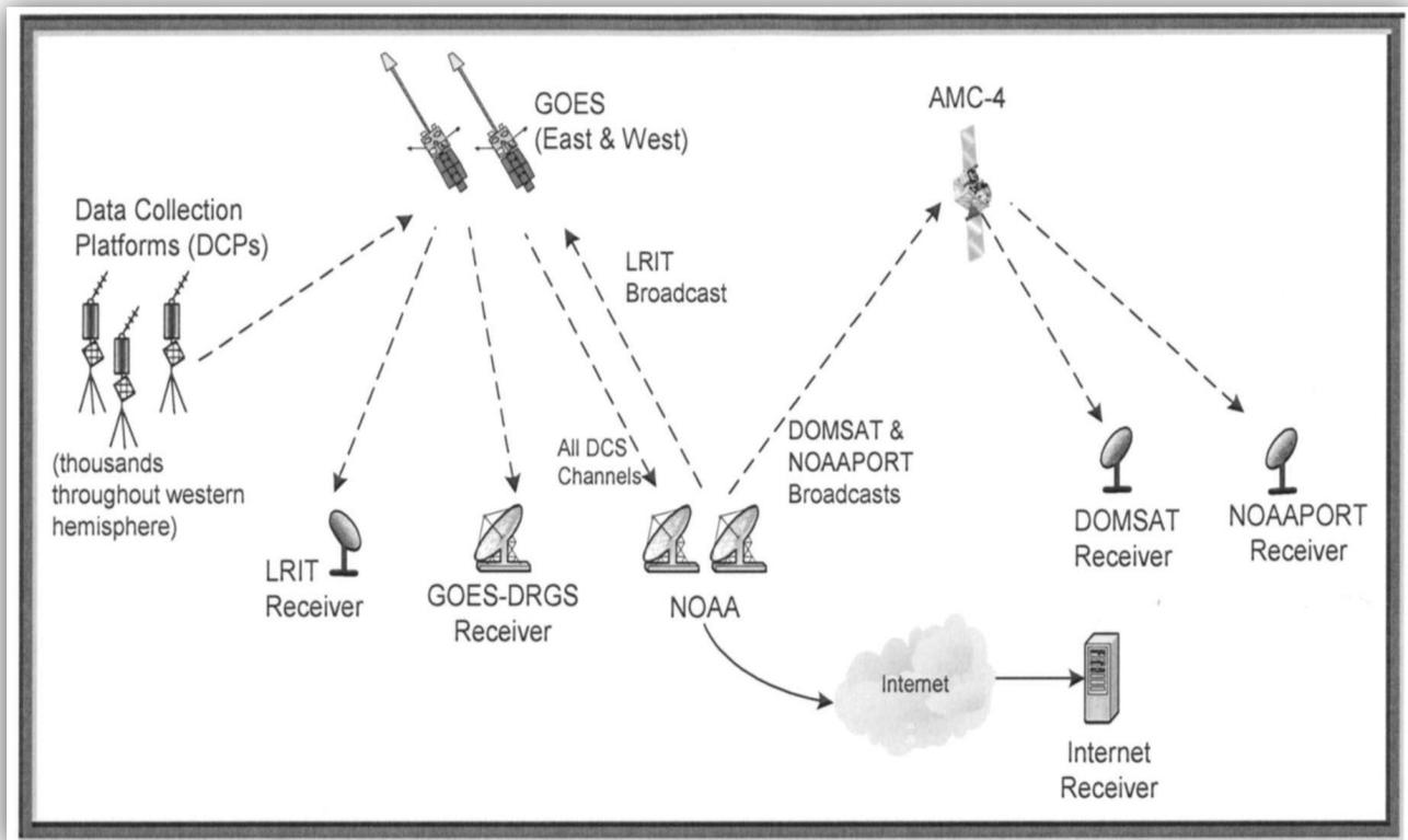
**Figure 5-3. Typical Configuration of the GOES System**
