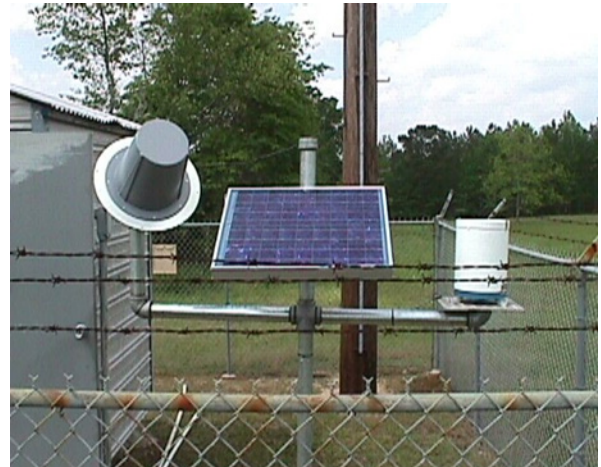
Figure 5-2 Typical Field Installation of a Precipitation Gage
