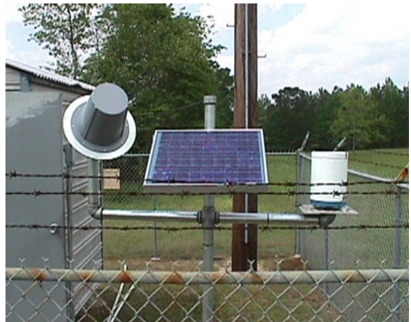
Figure 5-2 Typical Field Installation of a Precipitation Gage
