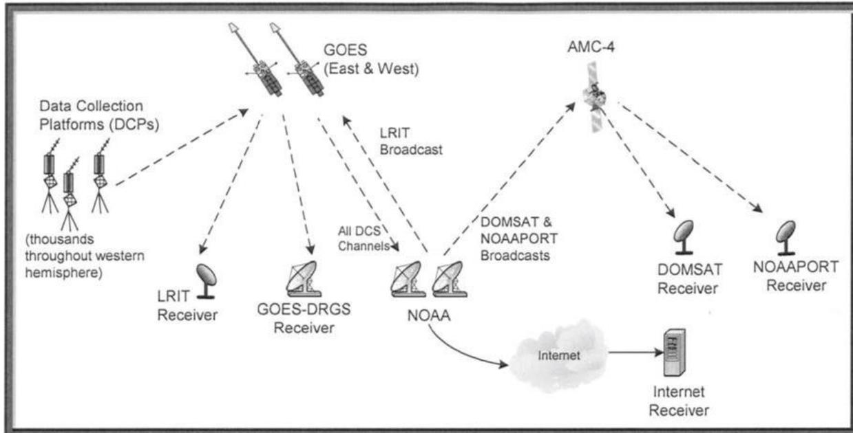
**Figure 5-3 Typical configuration of the GOES System**
