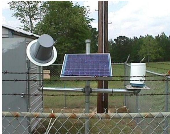
**Figure 5-2 Typical Field Installation of a Precipitation Gage**
