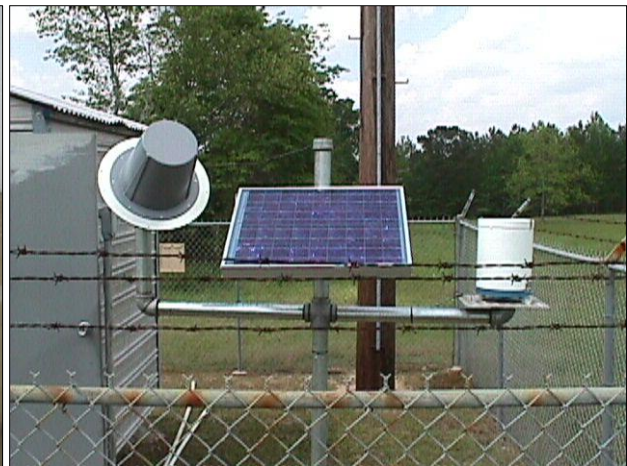
Figure 5-2 Typical Field Installation of Precipitation Gage
