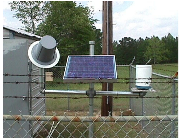
Figure 5-2 Typical Field Installation of a Precipitation Gage
