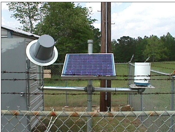
Figure 5-2 Typical Field Installation of Precipitation Gage
