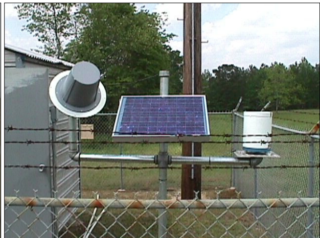
Figure 5-2 Typical Field Installation of Precipitation Gage
