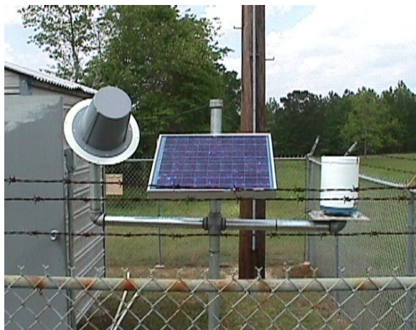
Figure 5-2 Typical Field Installation of a Precipitation Gage
