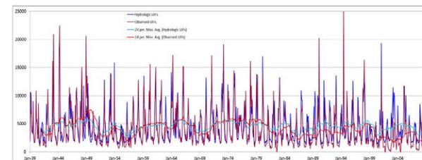
Figure 3.8.10: Hydrologic model results comparing USACE (observed; red) and hydrologic (based on the GWRI hydrologic model; blue) unimpaired flows. Starting in the 1980s, the observed UIFs are increasingly drier (up to 2,500 cfs) than the hydrologic UIFs, with low flows more severely affected.
