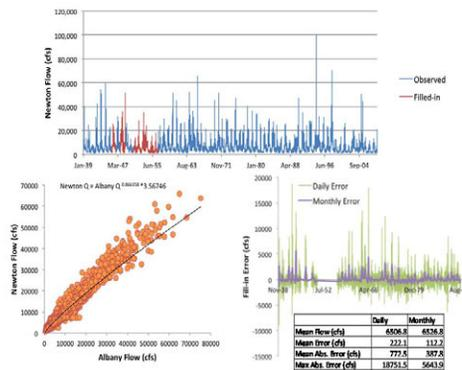
Figure 3.13.4: Estimation of Newton node streamflows.
