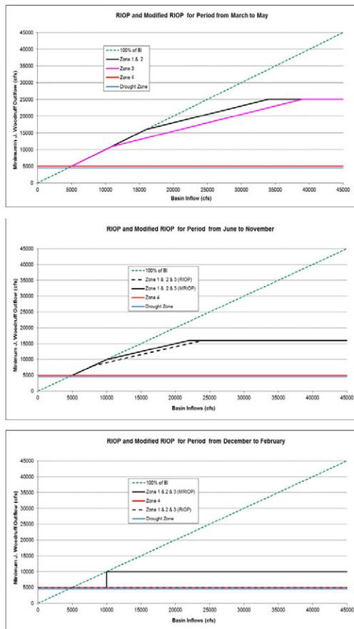
Figure 4.2.5: Comparison between the J. Woodruff minimum discharge requirements for the current (RIOP) and improved or modified RIOP (MRIOP) operations sets.
