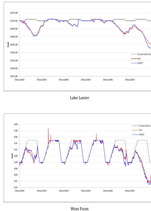
Figure 4.3.1: Daily reservoir elevation sequences for Lakes Lanier and West Point corresponding to the current operational procedures.
