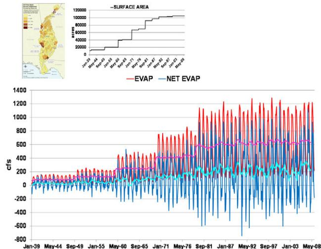
Figure B.2: Monthly evaporation and net evaporation, and associated 12-month moving average sequences from ACF impoundments (other than main stem reservoirs).
