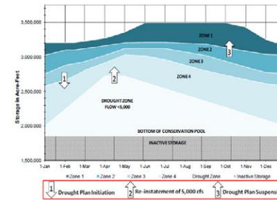
Figure 4.2.4: Composite reservoir storage zones under the improved operational procedures (USACE, 2012). The Composite storage is the sum of the storages at Lakes Lanier, West Point, and W.F. George.
