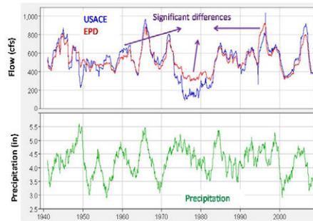
Figure 3.13.3: Two year moving averages of unimpaired flows and precipitation in the Newton reach.
