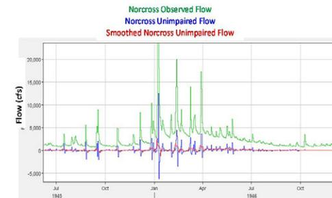
Figure 3.2.5: Negative unimpaired flows resulting during periods of high streamflow.
