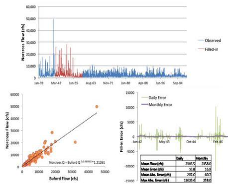
Figure 3.2.4: Estimation of Norcross node streamflows.
