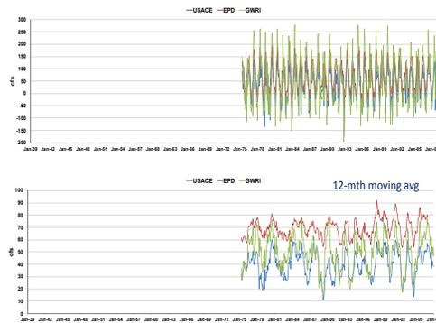
Figure 3.5.9: Net evaporation flows out of West Point Lake.
