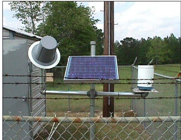
Figure 5-2. Typical Field Installation of a Precipitation Gage
