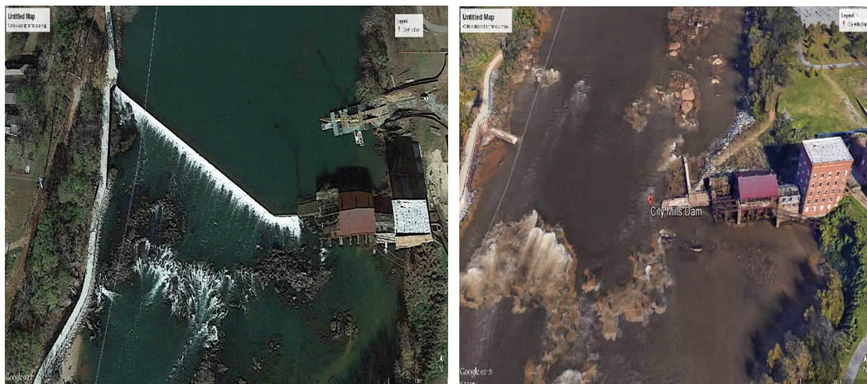
Figure 4-16. City Mills Dam Before and After Dam Removal (Photographs courtesy of Google Earth)
