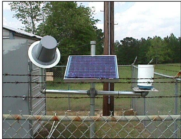
Figure 5-2. Typical Field Installation of a Precipitation Gage
