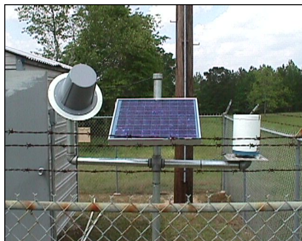
Figure 5-2. Typical Field Installation of a Precipitation Gage
