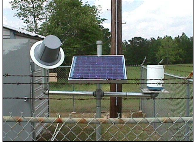
Figure 5-2. Typical Field Installation of a Precipitation Gage
