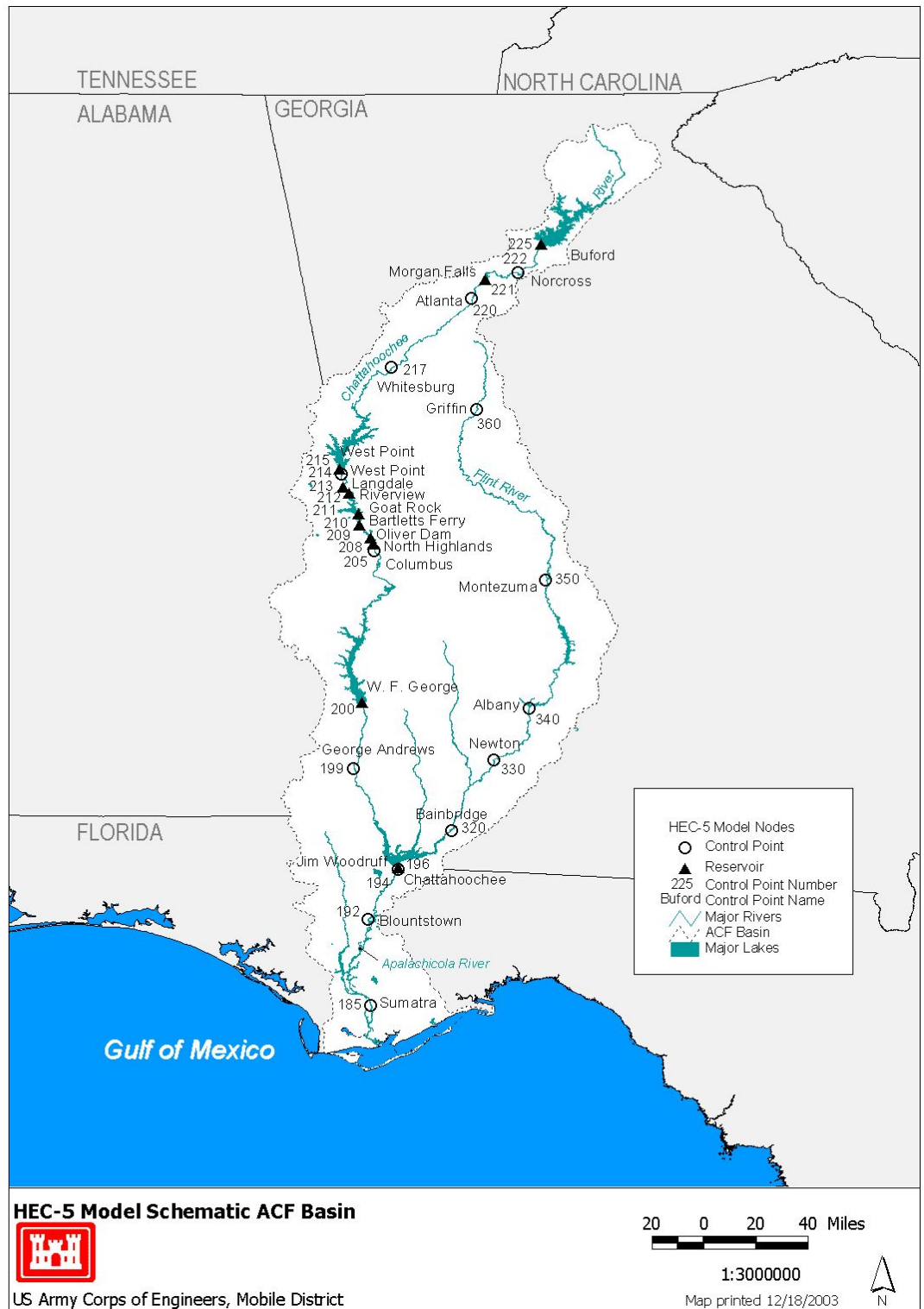
Figure 3. ACF basin schematic showing reservoirs and model computation points
