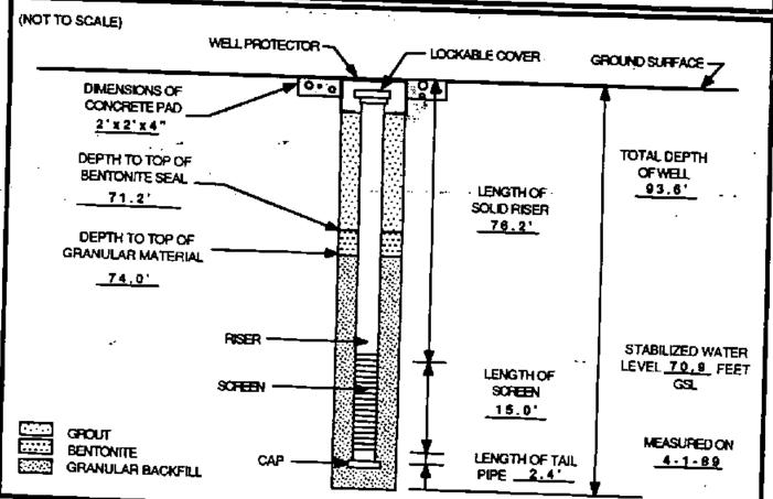
INSTALLED BY: \_\_ J. CRAWFORD INSTALLATION OBSERVED BY: \_\_ QA / QC **FWT** DISCREPANCIES: \_ NONE
