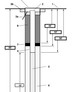
Note: Diagram not to scale. Depth reached 86', then backfilled with bentonite to 69'.
