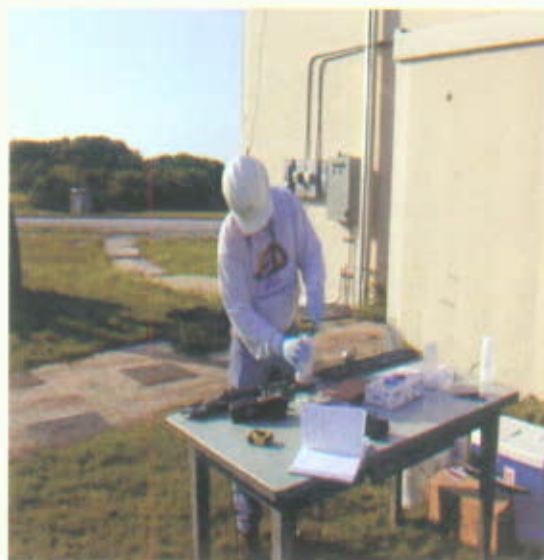
FIGURE 2. A soil sample being collected from along the length of the core into a bottle containing methanol.
