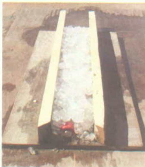
FIGURE 1. A soil core capped and cooling in an ice bath. The thermometer is visible in the end cap.
