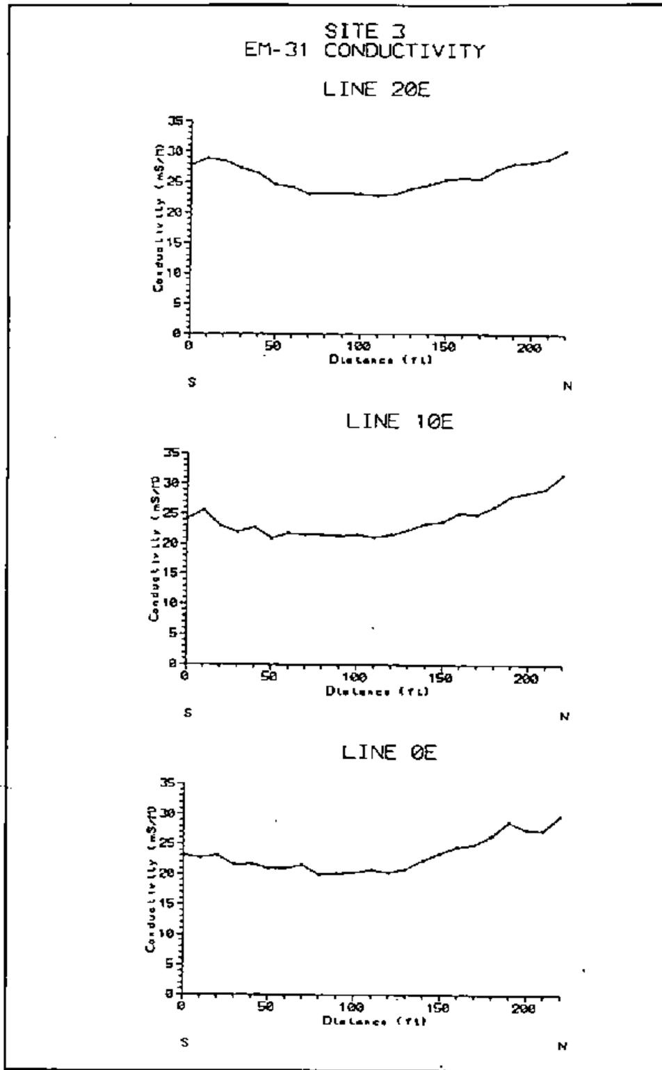
Figure 31. Results of EM-31 conductivity survey, Site 3
