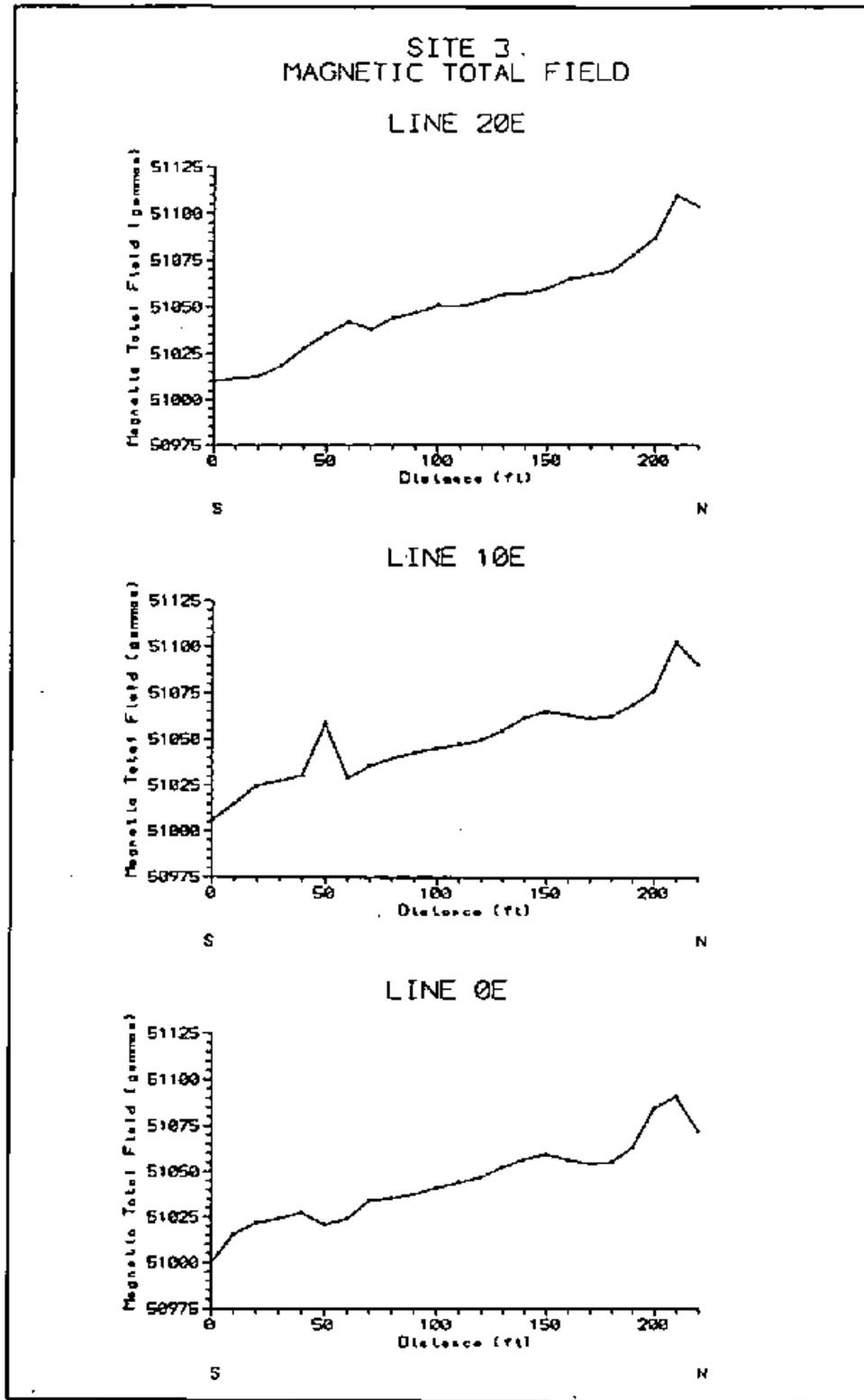
Figure 29. Results of magnetic total field survey, Site 3
