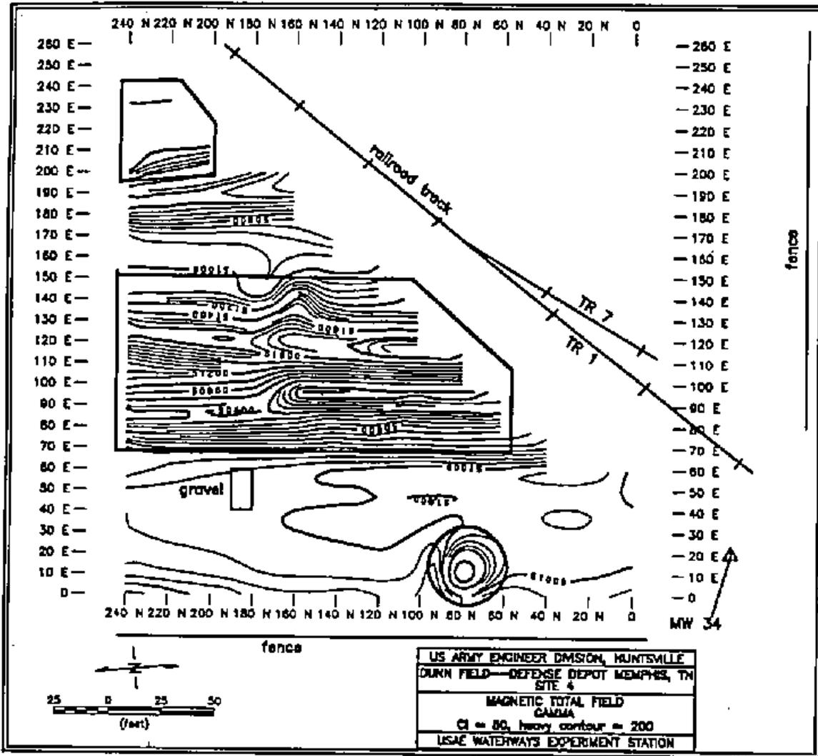
Figure 34. Results of magnetic total field survey, Site 4
