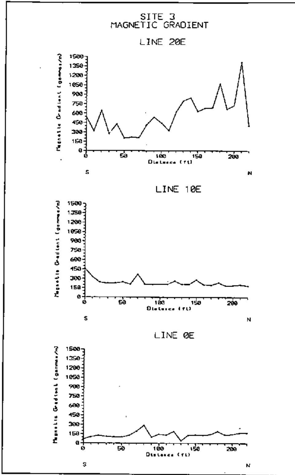
Figure 30. Results of magnetic gradient survey, Site 3
