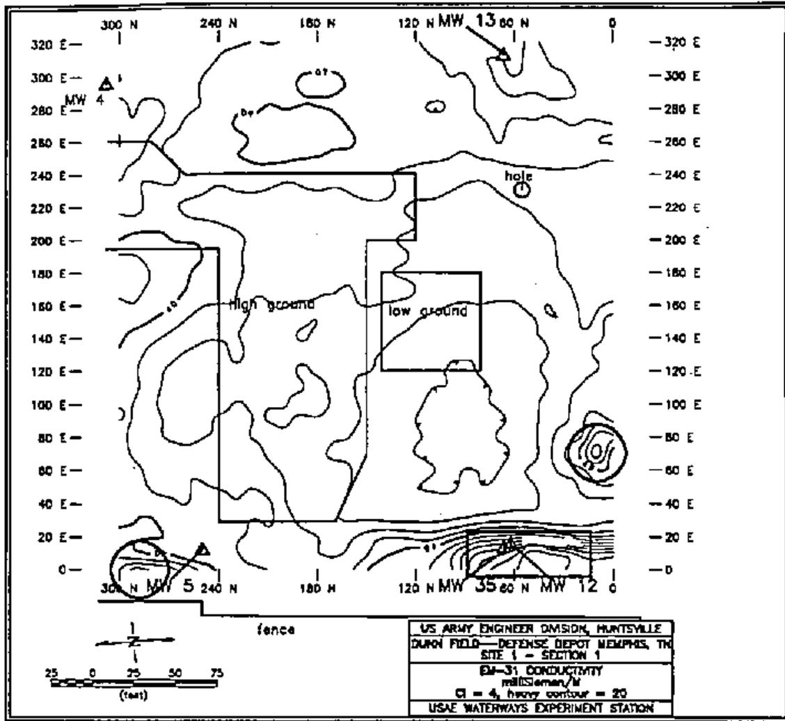
Figure 13. Results of EM-31 conductivity survey, Site 1, Section 1
