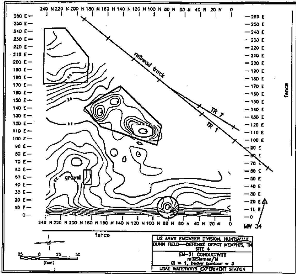
Figure 36. Results of EM-31 conductivity survey, Site 4
