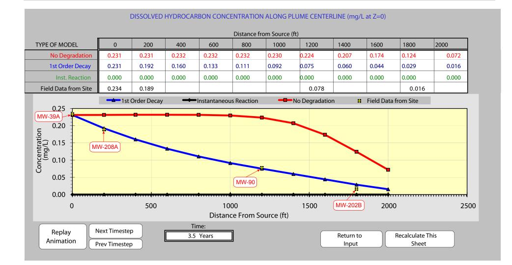
FIGURE 11 Attenuation Rate Calibration with Field Data for PCE Contaminant Plume Modeling Report, January 2009 Main Installation Defense Depot, Memphis, Tennessee
