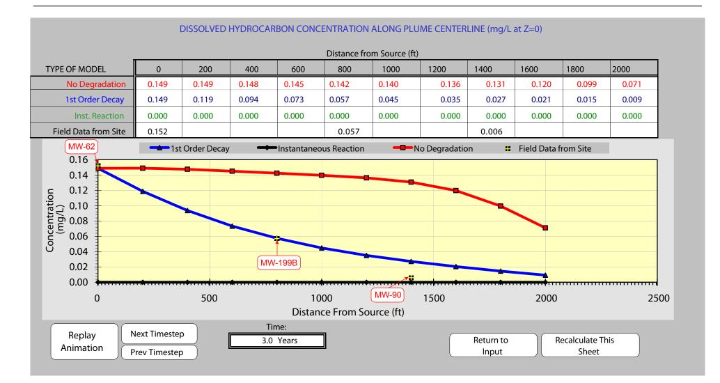
FIGURE 12 Attenuation Rate Calibration with Field Data for TCE Contaminant Plume Modeling Report, January 2009 Main Installation Defense Depot, Memphis, Tennessee
