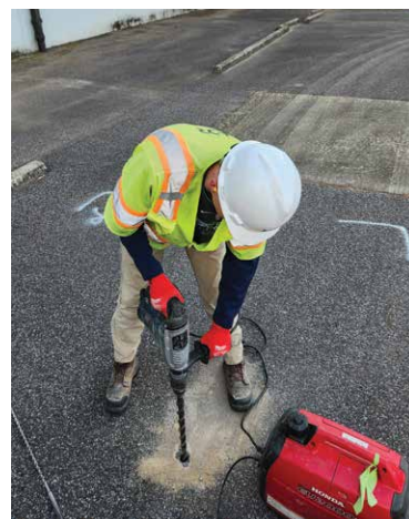
Matt Barickman, HDR geologist, drilling a hole through the pavement to collect a soil vapor screening sample for the Main Installation vapor intrusion study.
