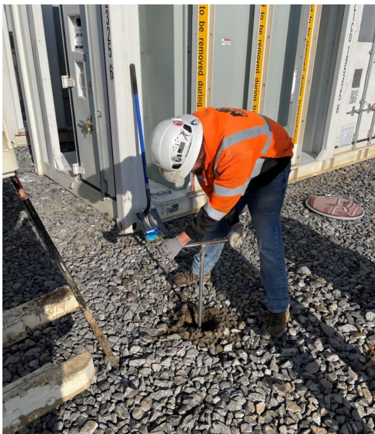
Photograph B-9. Hand Augering at DDMT-873-02
