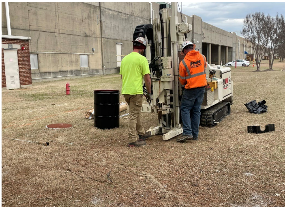
Photograph B-4. DPT Drilling at DDMT-550-01
