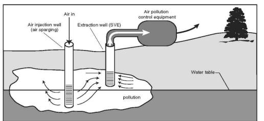
The air sparging or AS portion of the AS-SVE process involves the injection of air or oxygen through a contaminated aquifer. Injected air removes volatile and semi -volatile organic contaminants by volatilization. The injected air helps to flush the contaminants into the unsaturated zone.
