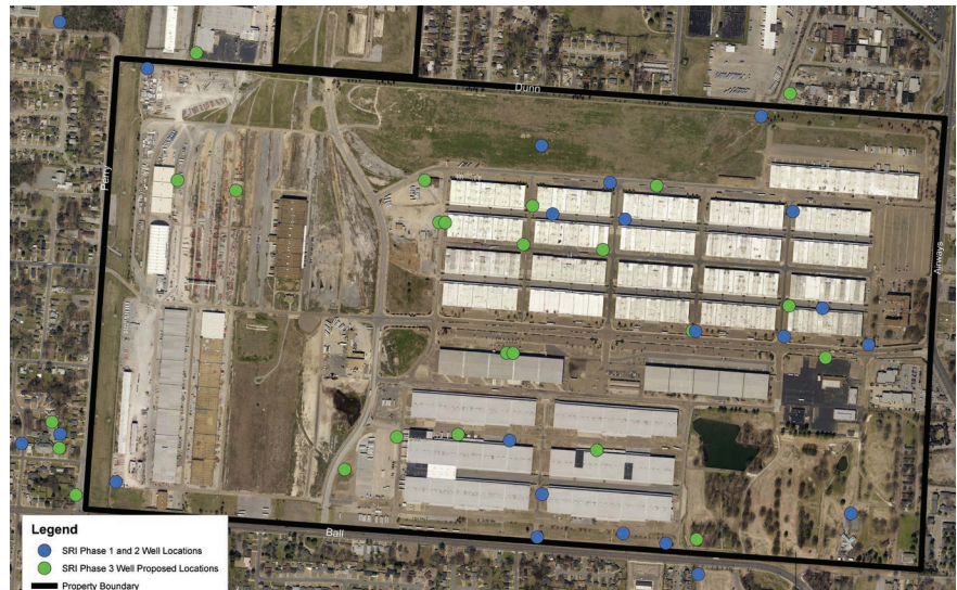
The Army will continue the Supplemental Remedial Investigation by installing Phase 3 monitoring wells (green dots) in 2018. The Phases 1 and 2 monitoring wells (blue dots) were installed in 2015 through April 2017.
