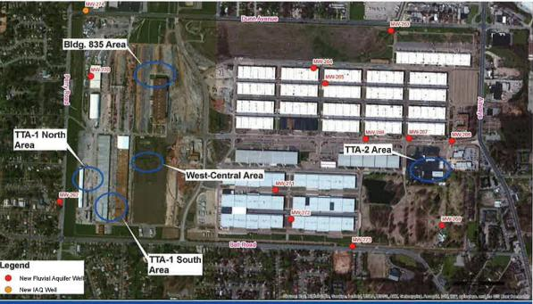
Enhanced bioremediation treatment was performed at five areas on the Main Installation. An additional investigation scheduled to begin in 2015 will install 13 monitoring wells, identified by the colored dots.
