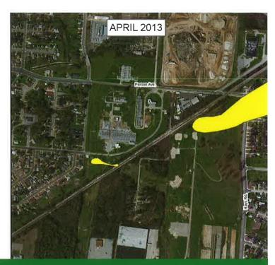
The area of groundwater contamination above 50 ppb is shown by yellow shading. From 2007 through 2013, the Dunn Field and Off Depot cleanup actions succeeded in shrinking the area of groundwater above the cleanup goal. TDEC is investigating for off site sources of groundwater contamination that is moving across the north part of Dunn Field.
