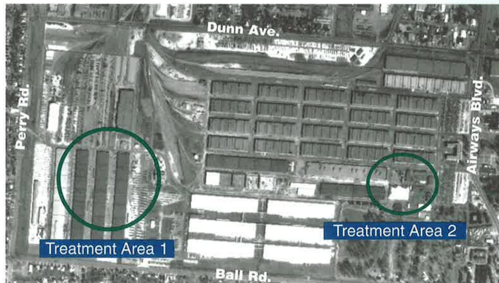
This aerial photo of the Main Installation identifies the two areas where Enhanced Bioremediation Treatment (EBT) will be used to treat groundwater in the shallow aquifer beneath the Main Installation.
