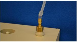
Figure 5. VAPOR PIN<sup>®</sup> sample connection
