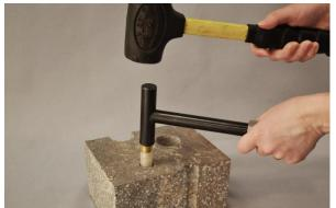
Figure 2. Installing the VAPOR PIN®
