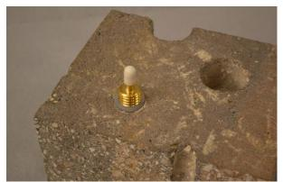
Figure 3. Installed VAPOR PIN®
