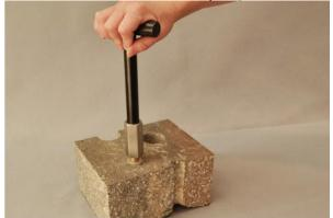
Figure 7. Removing the VAPOR PIN®
