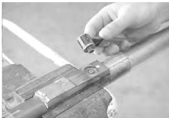
Figure 8.1: Unthread the membrane from the probe block.
