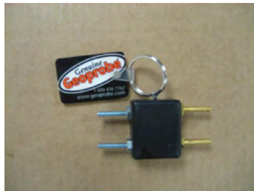
Figure 5.9: EC Dipole Test Jig
