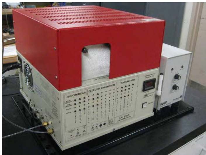
Figure 1: GC1000: SRI 310GC with XSD Controller
