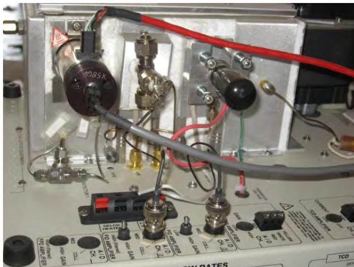
Figure 2: GC Detectors – left to right - XSD, FID, PID
