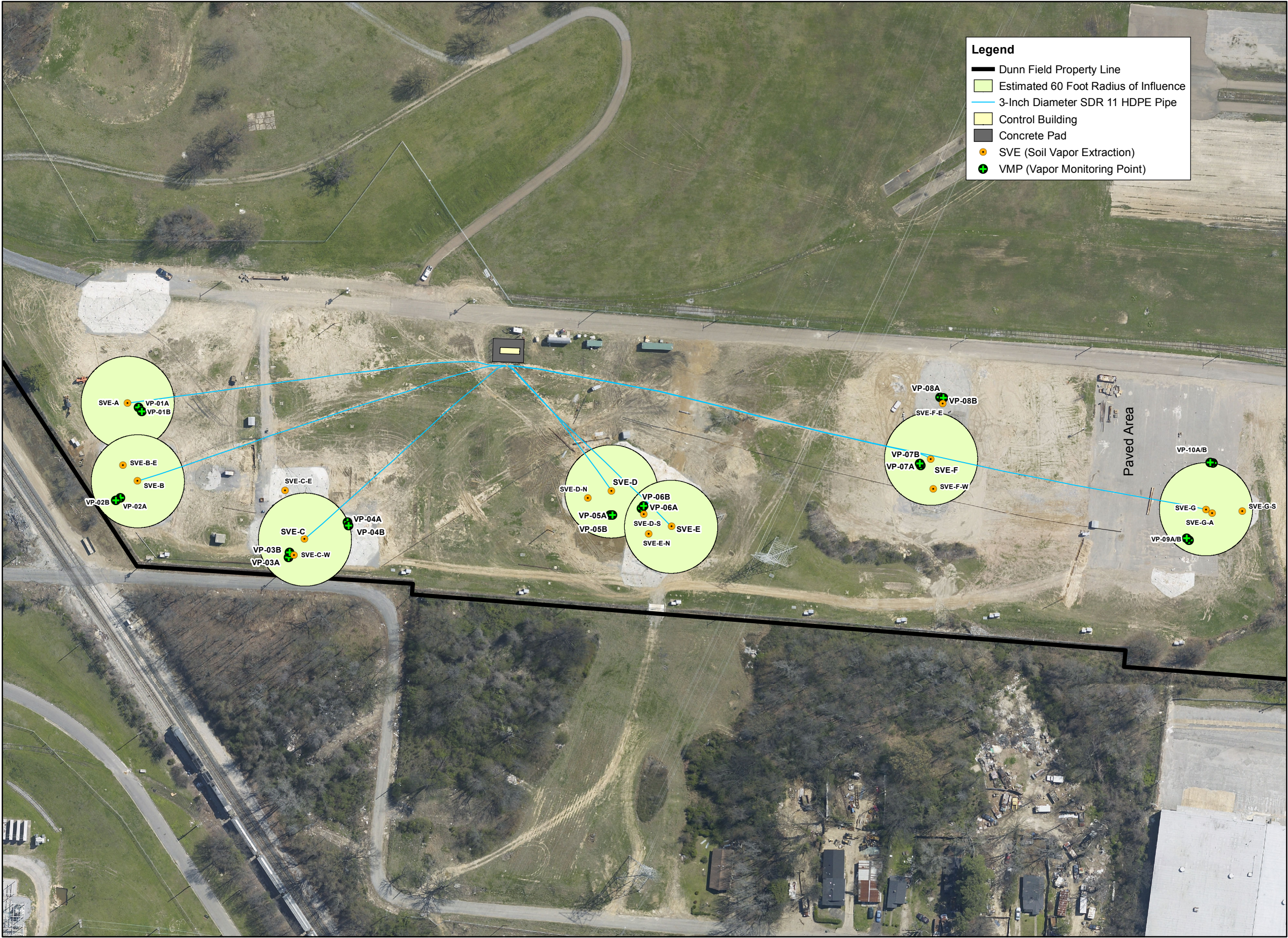
Figure 16 FLUVIAL SVE SYSTEM
