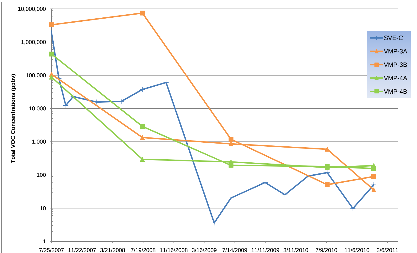
Figure 8 TREND OF TOTAL VOC CONCENTRATIONS AT TA-1E SVE WELL AND VMPs REBOUND TEST AND CONFIRMATION SOIL SAMPLING FLUVIAL SOIL VAPOR EXTRACTION SYSTEM Dunn Field - Defense Depot Memphis, Tennessee
