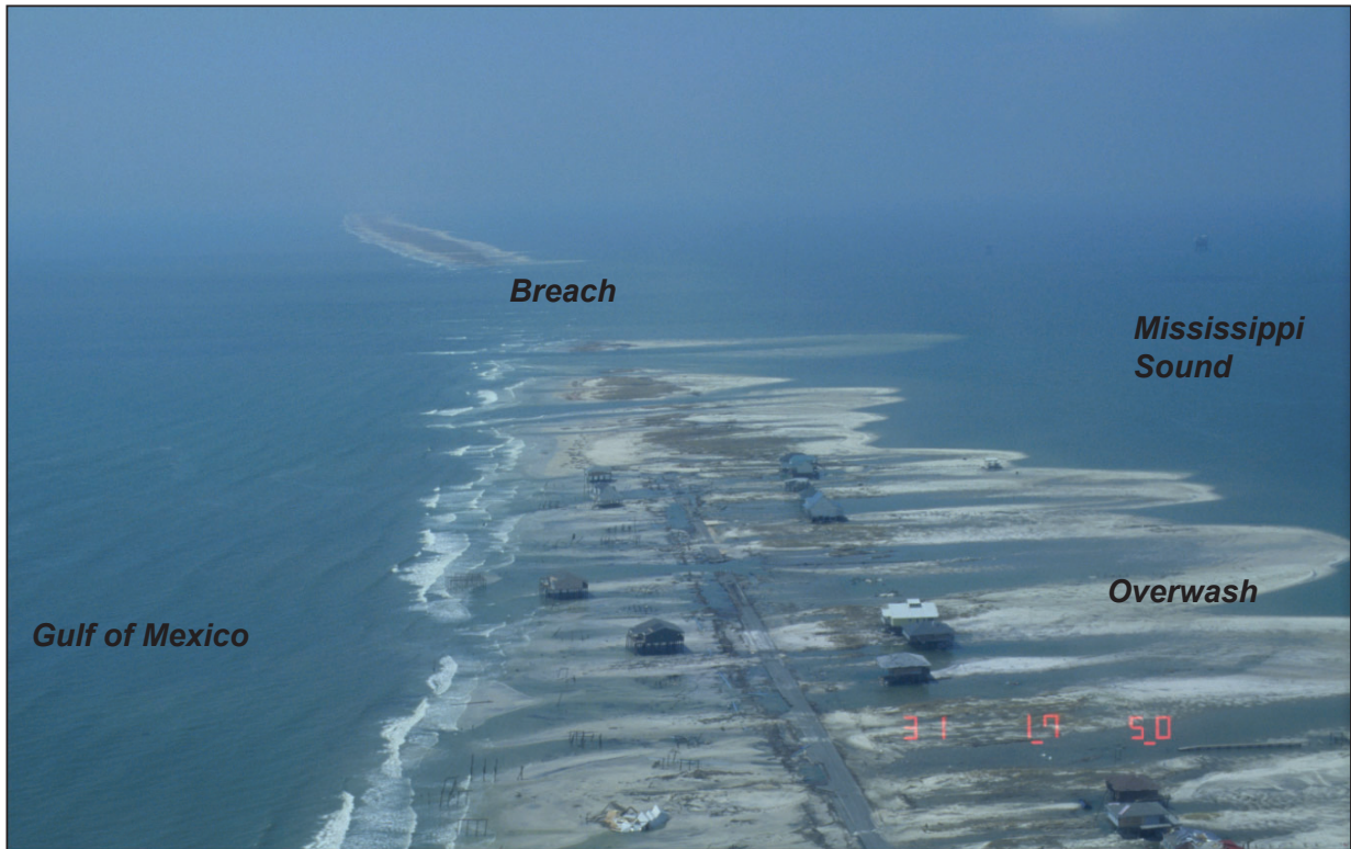
Figure 2. Extensive shoreline erosion, overwash, breaching, and damage to the infrastructure at Dauphin Island during Hurricane Katrina in 2005. The view is of the central portion of the island looking west. The image was taken August 31, 2005, U.S. Geological Survey post-storm aerial oblique photography ( https://coastal.er.usgs.gov/hurricanes/katrina/post-storm-photos/obliquephotos.html ).
